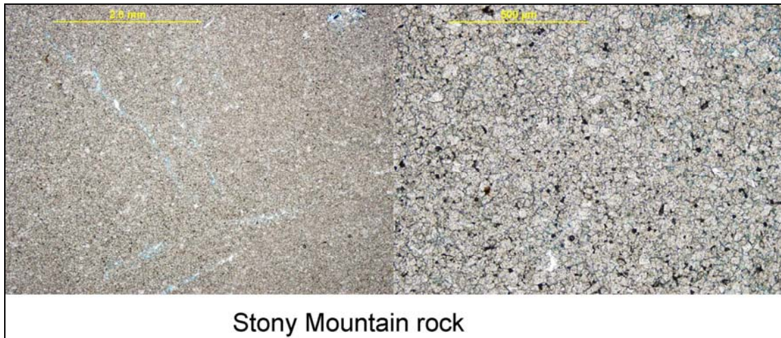
Figure 29. Thin section of Stony Mountain dolomite.
