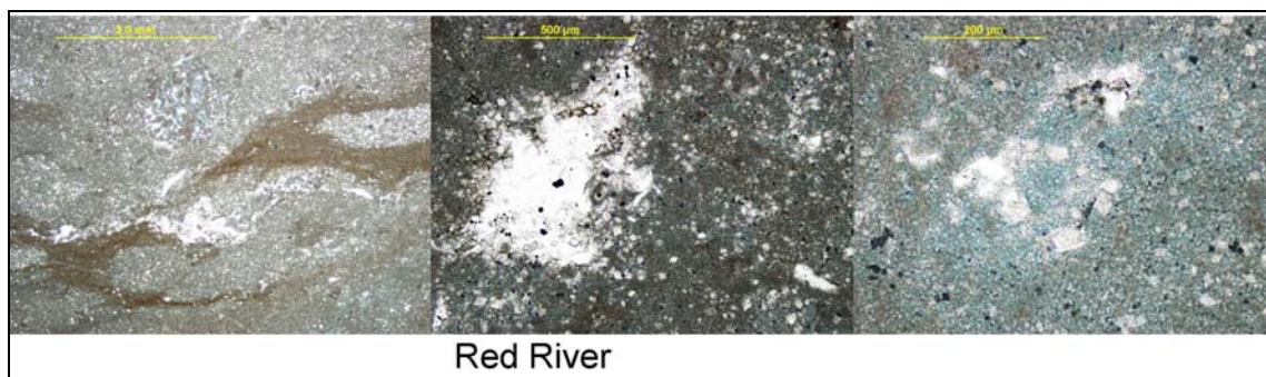
Figure 30. Thin section of Red River dolomite.
