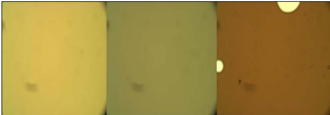
Figure 26. Left to right 80, 50, and 20% 1-methylnaphthalene added to Stony Mountain crude oil.
