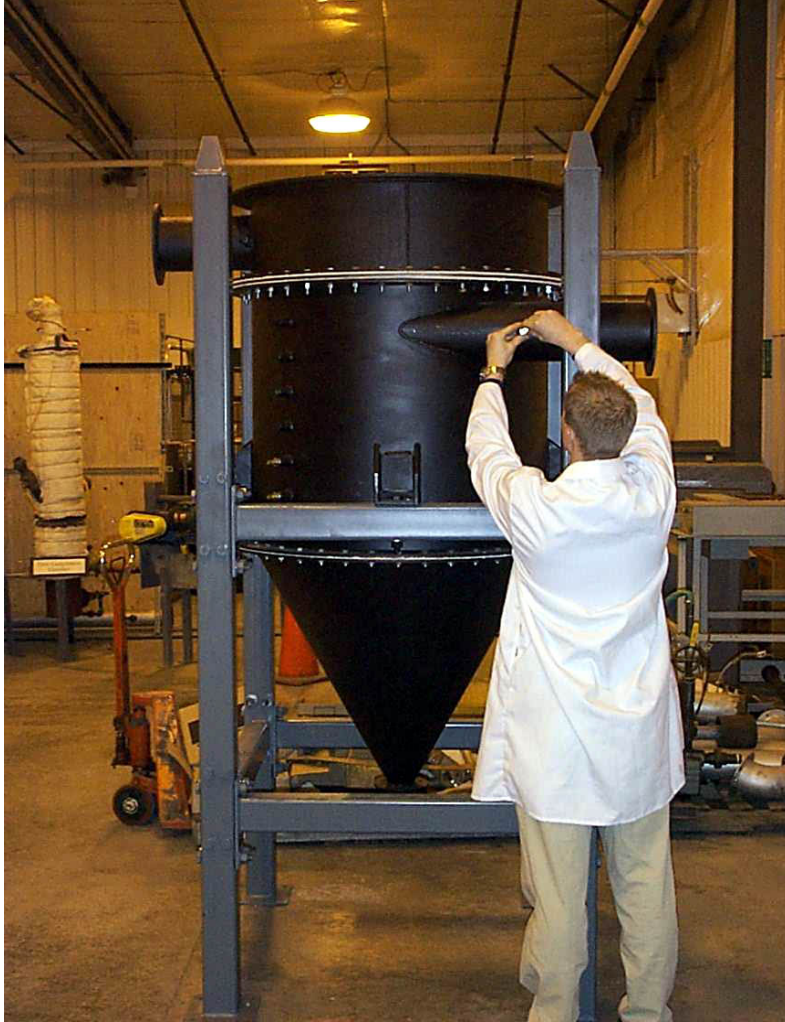
Figure 7 Photographs of the moving bed granular filter (a) after construction, (b) after installation
