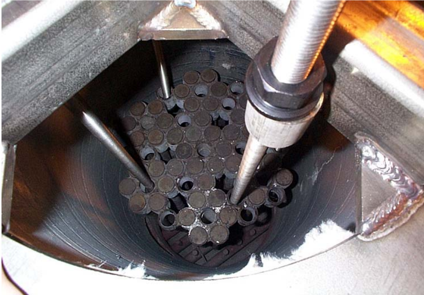
Figure 5 Overhead view of latent heat ballast system installed in 5 tpd biomass gasifier
