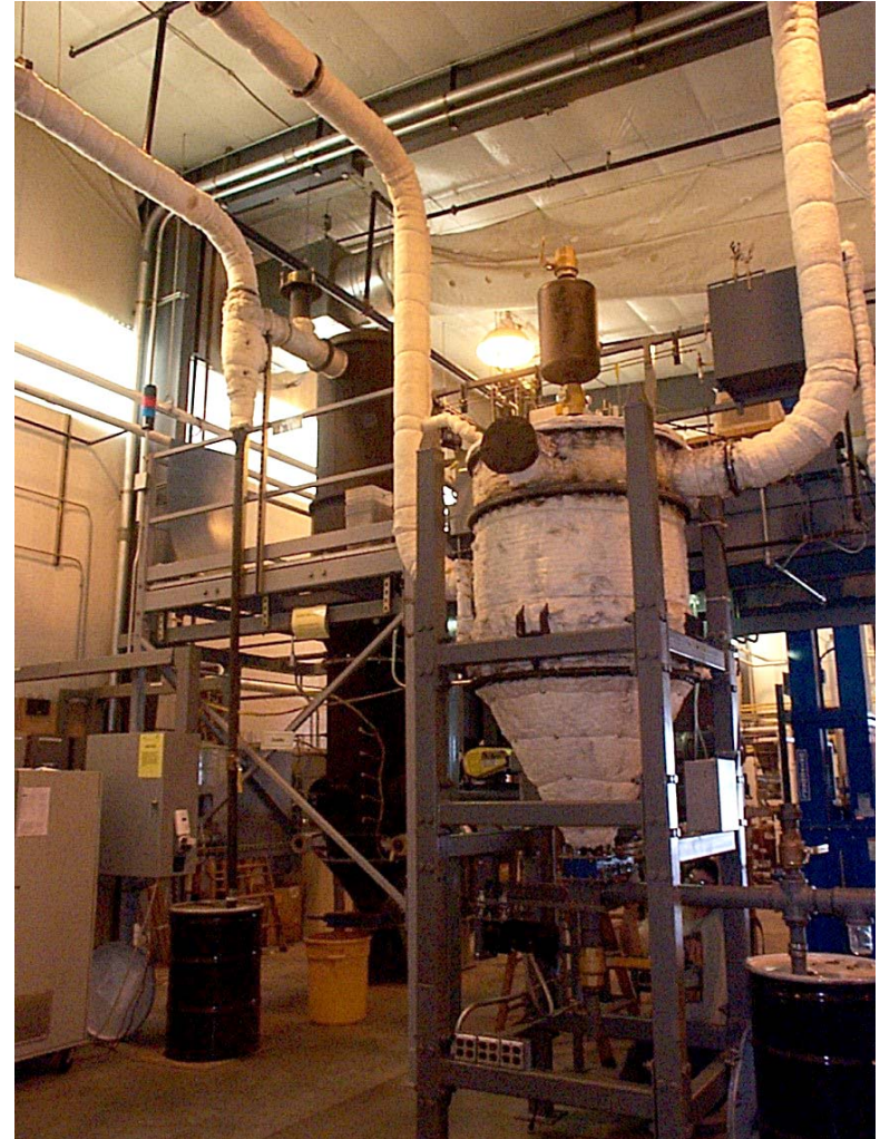
Figure 7 Photographs of the moving bed granular filter (a) after construction, (b) after installation
