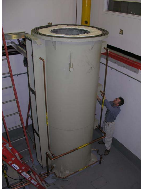
Figure 9. Production-scale CWF furnace.
