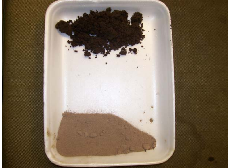
Figure 2. Crushed core before (top) and after (bottom) 200 psig experiment with Oman oil.
