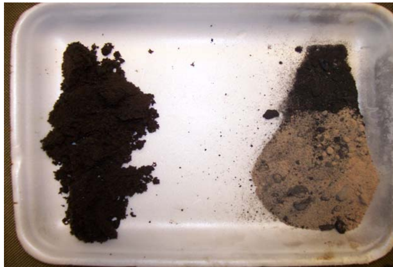
Figure 3. Crushed core before (left) and after (right) 50 psig experiment with Oman oil.
