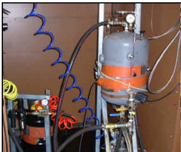
Figure 6. Spinner II Model 60 Centrifuge Experimental Setup.
