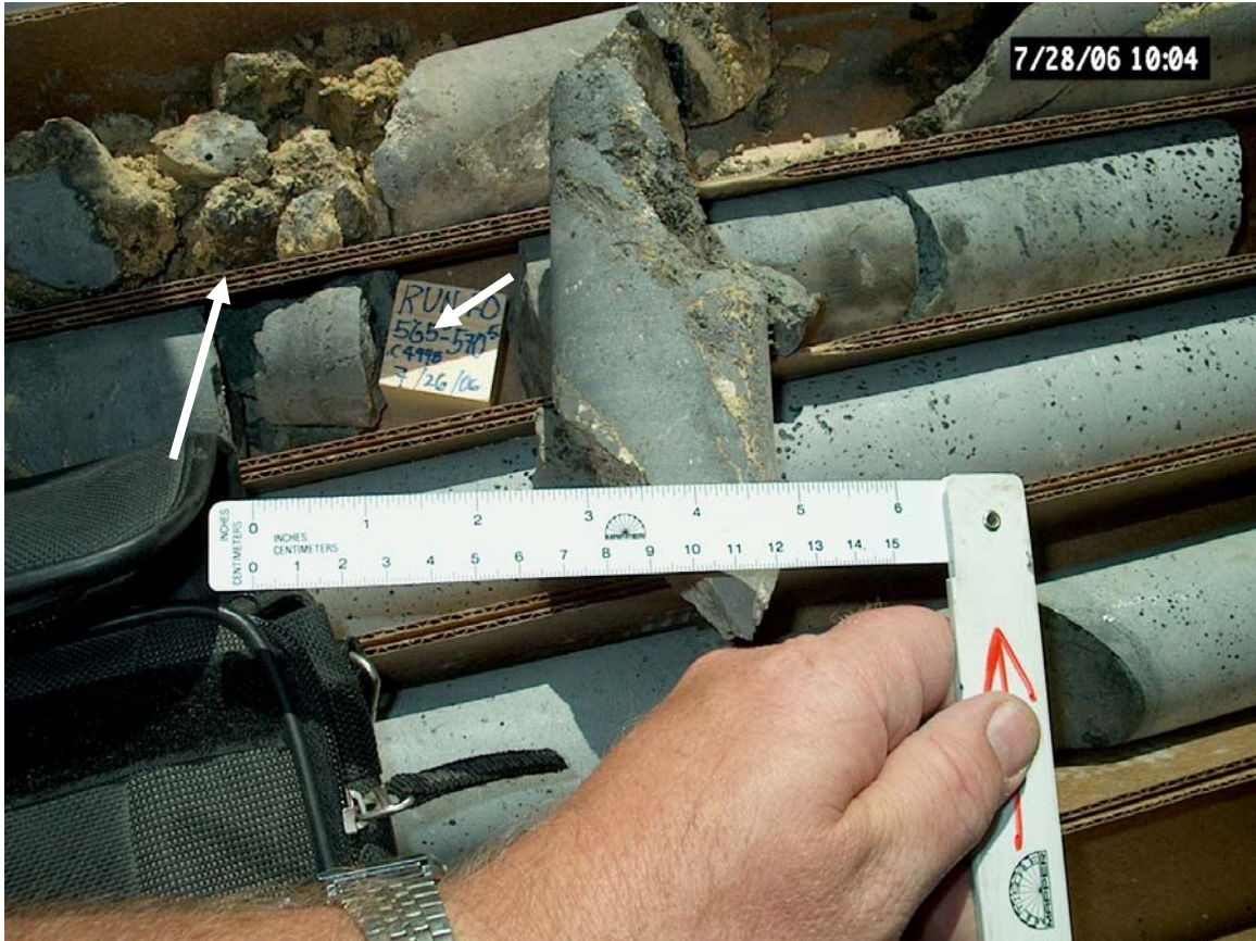
Figure 6.14. High-Angle Fractures Bounding Basalt Breccia and Opaline Matrix at 563.8 ft bgs in Core Hole C4998
