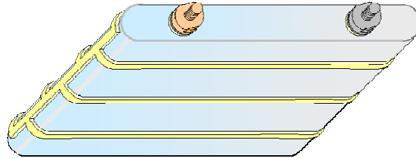
Fig. 10. Rigid Cell with Sleeve that Provides Cooling Passages between Adjacent Cells
