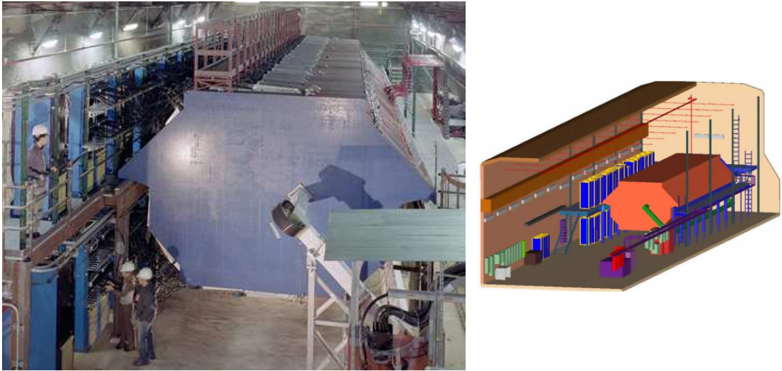
Figure 3.13: MINOS Near Detector: Site and Photo.
