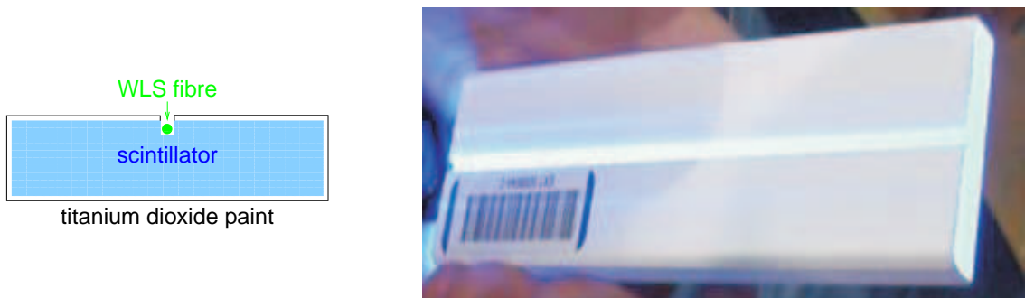
Figure 3.6: Scintillator Strip Diagram and Photo.
