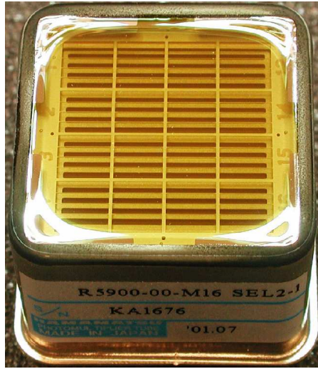
Figure 3.7: The MINOS Multi-Anode PMT.
