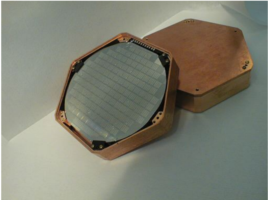
Figure 4.1: A Photograph of a ZIP detector in its Housing. The exposed face shows the phonon sensor pattern.
