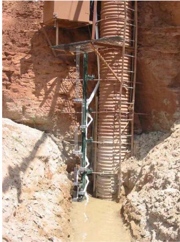
**Figure 5.2:** Close-up view of the TDR probe stack. Seven probes are visible with the top of the waveguides of the eighth probe barely visible at the water surface.
