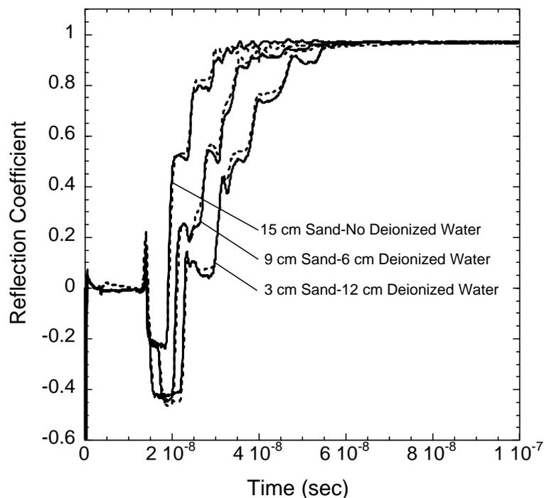
**Figure 3.2.** TDR traces measured in a layered sequence of sand and deionized water. Shown are traces for a probe submerged in water with accompanying water saturated sand depths of 3, 9, and 15 cm. The solid lines designate the measured traces while the dotted lines correspond to the modeled traces.
