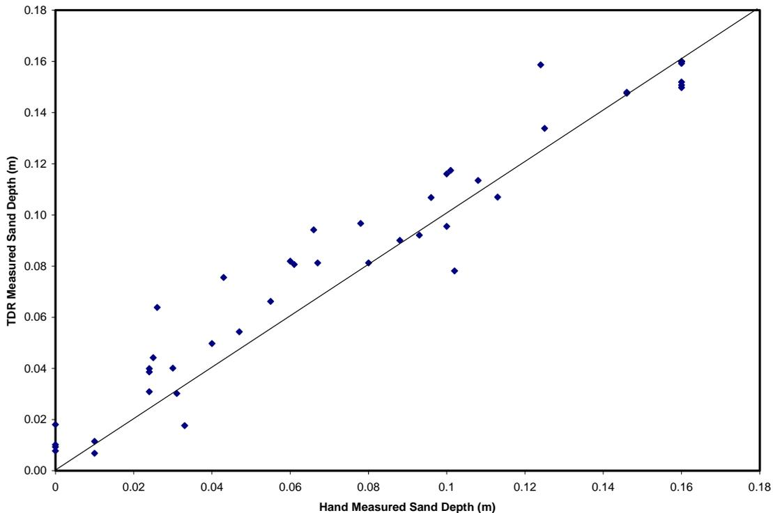
**Figure 4.7:** Scatter plot between sand depth measurements made by hand (see Figure 4.2) and those estimated from TDR traces. TDR traces were taken from the probes buried in the channel of the Rio Grande.
