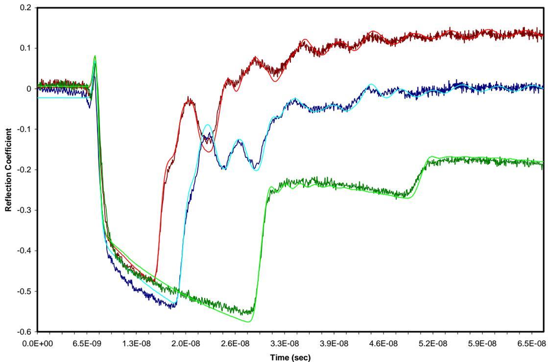
**Figure 4.4:** Three pairs of measured and modeled TDR traces. The measured trace is always the darker shaded line as well as shows high frequency noise, absent in the modeled traces. As the water depth increases the trace becomes broader and trace values decline at later times.
