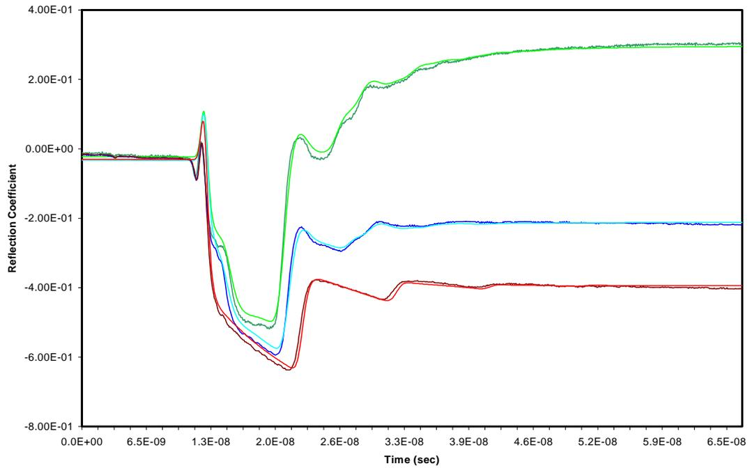
**Figure 4.9:** Three pairs of measured and modeled TDR traces. The measured trace is always the darker shaded line as well as shows high frequency noise absent in the modeled traces. Trace narrows as sand replaces water along the probe.
