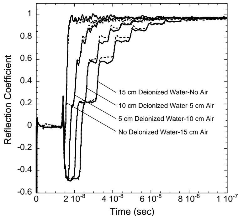
**Figure 3.1.** TDR traces measured with a varying depth of deionized water along the length of the probe. Shown are traces for water depths of 0, 5, 10, and 15 cm. The solid lines designate the measured traces while the dotted lines correspond to the modeled traces.
