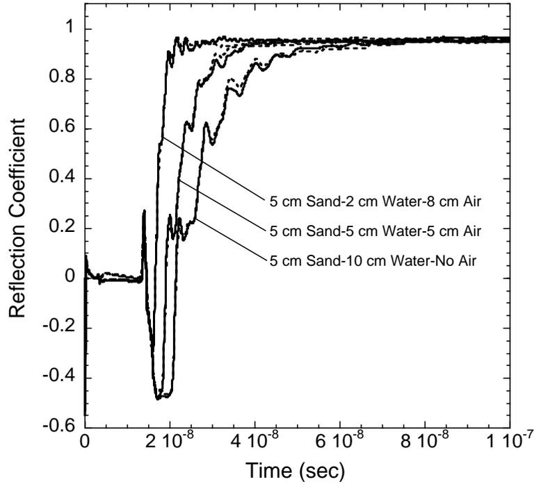
**Figure 3.3.** TDR traces measured in a layered sequence of sand, deionized water, and air. Shown are traces for a 5 cm depth of saturated sand and increasing depth of water. The solid lines designate the measured traces while the dotted lines correspond to the modeled traces.
