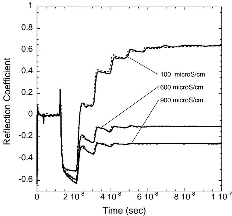
**Figure 3.4.** TDR traces measured with varying conductivity. Shown are traces for conductivities of 100, 600, and 900  $\mu\text{S}/\text{cm}$ . The solid lines designate the measured traces while the dotted lines correspond to the modeled traces.
