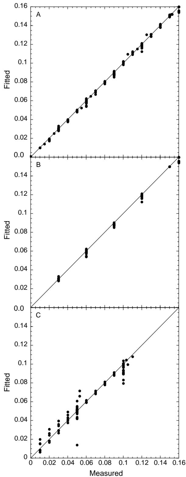
**Figure 3.5.** Scatter plots showing the difference between the actual interface location and that estimated with the multisection model. A) Scatter plot for all data from Tests 1, 2, and 3; B) scatter plot for all data from Test 6; and C) scatter plot for all data from Test 4. Plotted are the measured/modeled depths of water (m). The line plotted is for the 1:1 relation.
