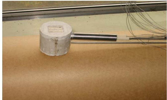
Figure 1 – Photo of an air-cooled probe showing wire leads connected to sensors and thermocouples and two lengths of 1/8 in stainless steel tubing for air inlet and outlet
