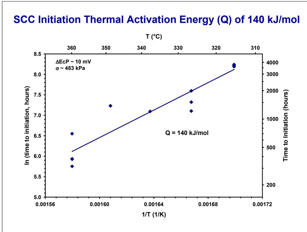
Tests were conducted at a constant electrochemical potential distance from the Ni/NiO phase transition in order to determine the activation energy for SCC initiation. The thermal activation energy (Q) for solution annealed Alloy 600 SCC initiation was determined based on testing at 360, 338, and 316°C. Q was determined to be 140 kJ/mol for the single Alloy 600 heat NX5805G.
