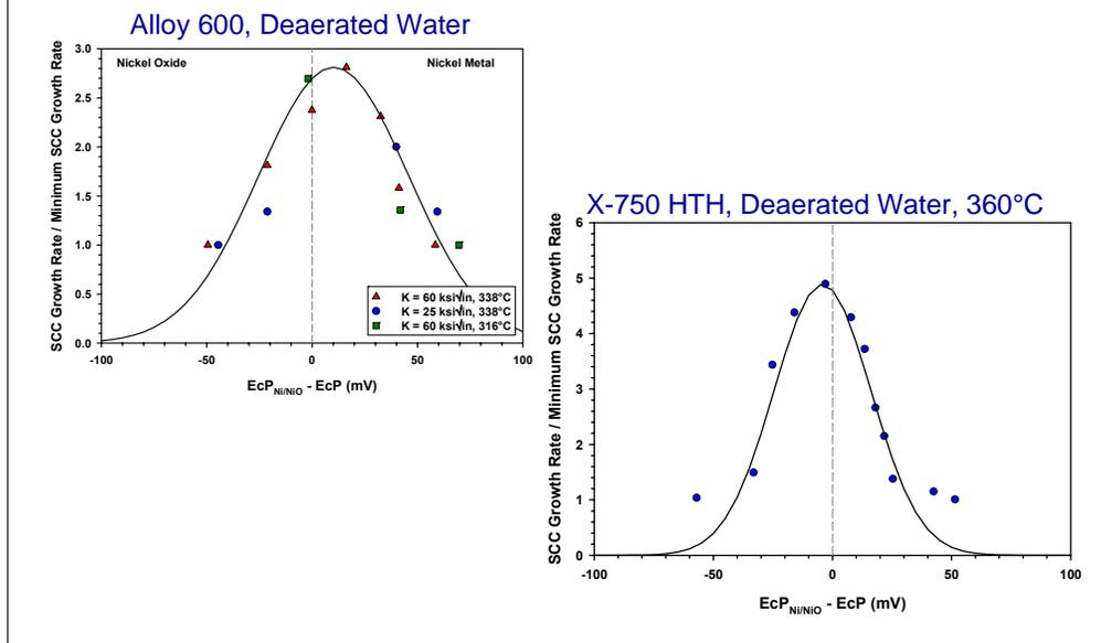
Previous testing has shown that SCC growth rates in Ni alloys exposed to high temperature, high purity water are affected by the Corrosion potential distance from the nickel oxide phase transition,  $\Delta EcP = (EcP_{Ni/NiO} - EcP)$ . This quantity describes, fundamentally, the coolant hydrogen crack growth rate functionality.
