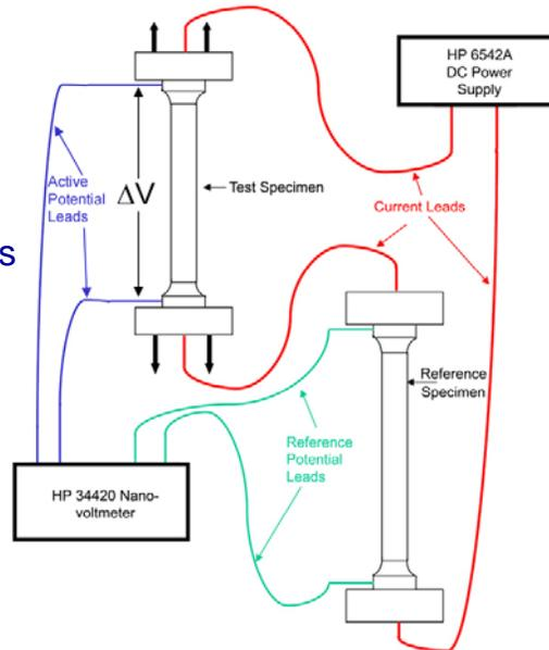
$\therefore$  Strain is related to change in resistance due to SCC initiation
