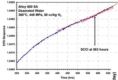
CT and metallography indicate 40 mils crack extension
