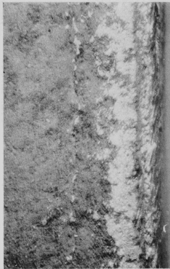
Figure 4. Magnified View of Plate No. 2 at Edge. Raised edge, parallel fissure, and adhering aluminum are seen clearly in this stereo.
