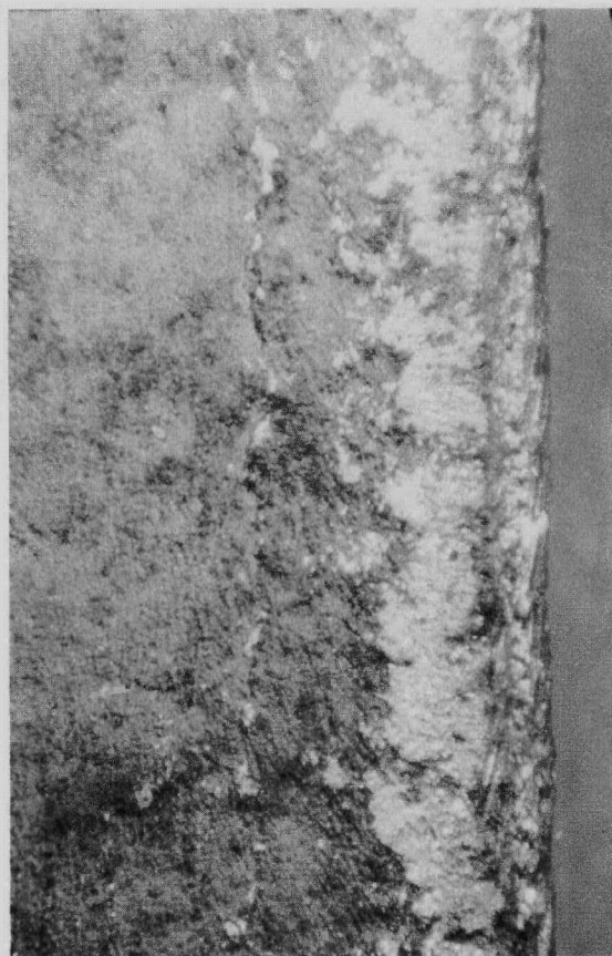
Figure 4. Magnified View of Plate No. 2 at Edge. Raised edge, parallel fissure, and adhering aluminum are seen clearly in this stereo.
