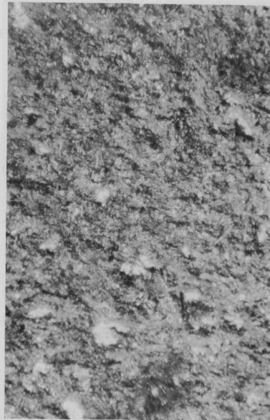
Figure 9. Typical View of Surface near Middle of Plate No. 5. Note evidence of poor contact between sheath and core.
