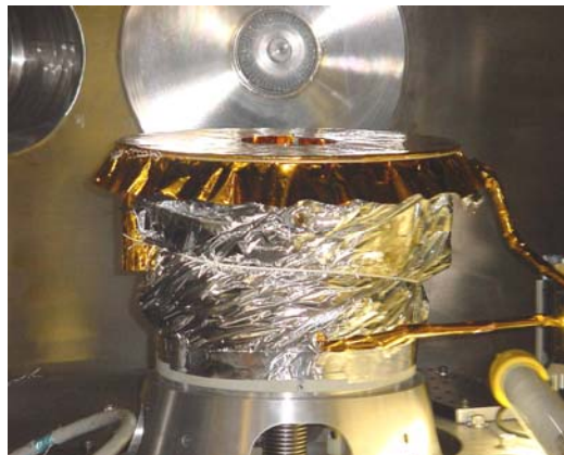
HTS Stability Bearing Cryostat Installed in DOE 10 kWh Flywheel
