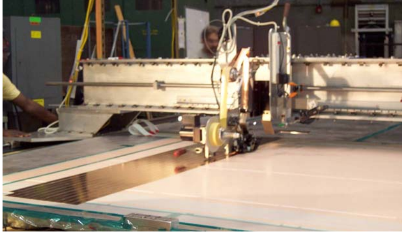
Fig. 6. Taping machine and carrier used for laying down the strips.
