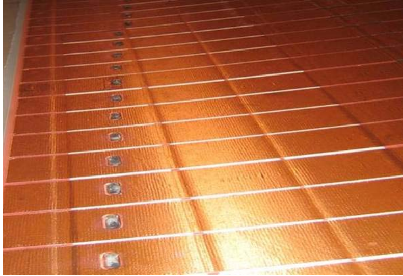
Fig. 7. The strips soldered to 16-channel cables after lamination. The three distinct white bands are the cables in the plane.
