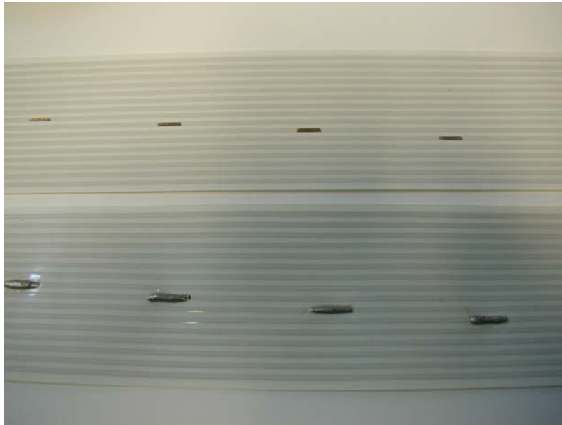
Fig. 4. 16-channel cable. The gap between the two pre-tinned channels matches the center of the adjacent strips.
