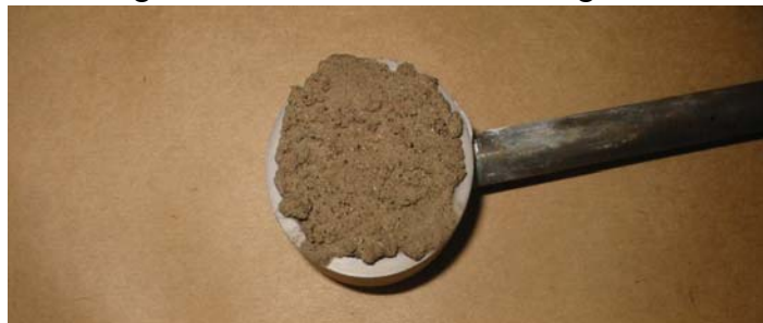
Figure 1 — ECR isothermal probe covered with ash.
