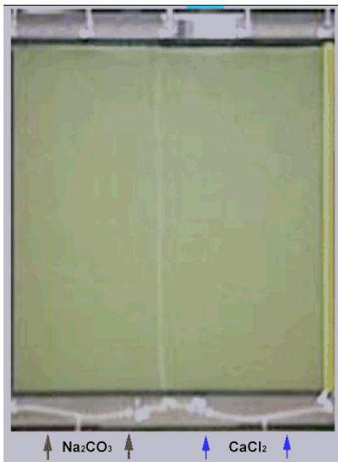
**Figure 1.** Mesoscale experimental flow cell (60 cm by 60 cm). The flow cell is filled with 0.5 mm quartz sand and is relatively thin in the third dimension. Two solutes are injected along two halves of the lower boundary as indicated by the red and blue arrows. The reaction causes precipitation of calcium carbonate minerals (the white zone approximately 0.5 cm wide in the center of the flow cell).
