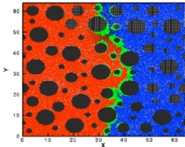
**Figure 2.** Pore-scale simulation of mixing of two solutes (blue and red) and reaction to form precipitated solid mineral (green). Details of the simulation method are provided in [8].
