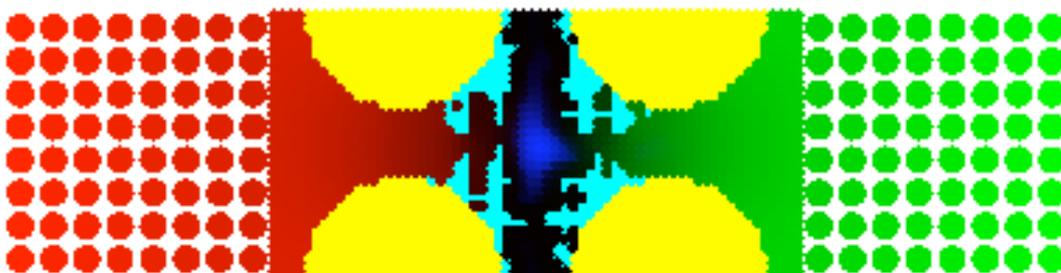
**Figure 3.** Visualization of hybrid simulation results at a single snapshot in time. The two diffusing and mixing solutes are represented by red and green (mixing into dark blues). Yellow indicates solid grains. Light blue represents precipitated mineral phases. The central portion is directly simulated at the pore scale whereas the outer zones are simulated using a continuum porous media approximation.
