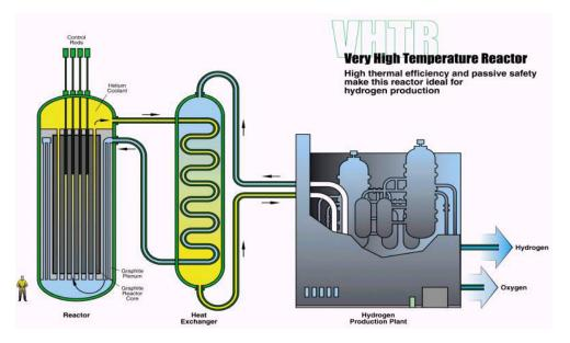
The reactor thermal power (400 - 600 MWt) and core configuration will be designed to assure passive decay heat removal without fuel damage during accidents. The fuel cycle will be a once-through, very high burnup, low-enriched uranium fuel cycle.
