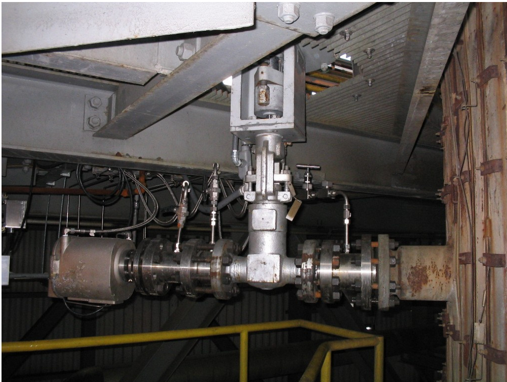
Figure 3. Pyrometer Optical Train Installed on Gasifier Nozzle
