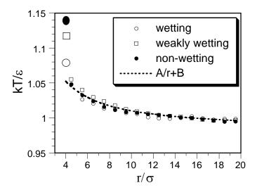
Figure 2: Radial temperature profiles from the simulations in which a single particle is heated by a constant heat source and the heat is removed from a spherical shell at distance  $20 \sigma$  away from the particle center. Presented data are for non-wetting, weakly wetting and wetting nanoparticles. Larger symbols represent temperatures of the particles. The dotted line is a fit to the T = A/r + B formula.
