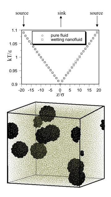
Figure 1: Bottom panel: A snapshot of atomic positions of the nanofluid model structure comprising of 8 crystalline nanoparticles embedded in a liquid. Top panel: Temperature profiles obtained from the heat source-sink simulations for pure melt and wetting particle nanofluid. The slope of the temperature profile allows determining thermal conductivity. The arrows indicate positions of the heat source and sink.
