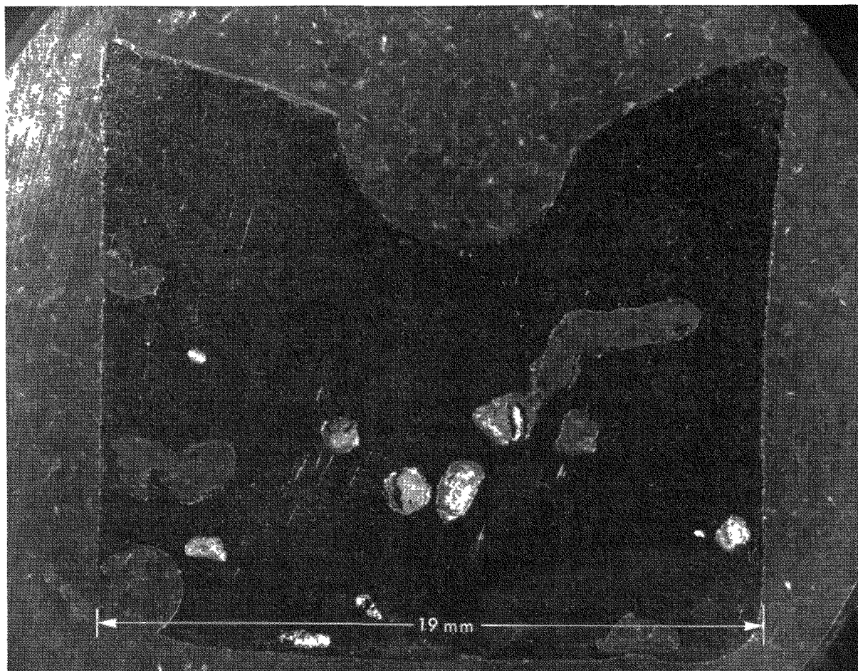
FIG. IV-6. Cross Section of Nickel Sample After Exposure to Steam at 1600°C for 90 min. (Exposed surface at top.)
