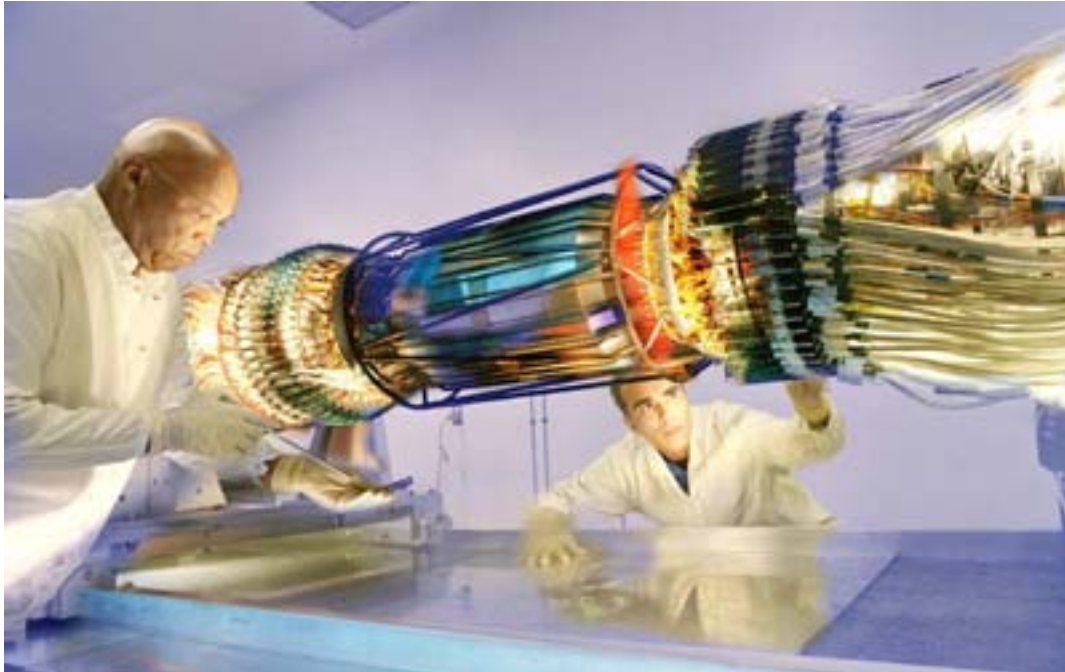
Figure I-1.5 The Silicon Vertex Tracker is at the heart of the BABAR experiment at SLAC. Its millions of sensitive elements typify the evolution of detector technology that is making experimental high-energy physics ever more data intensive. (Photo courtesy of Peter Ginter)
