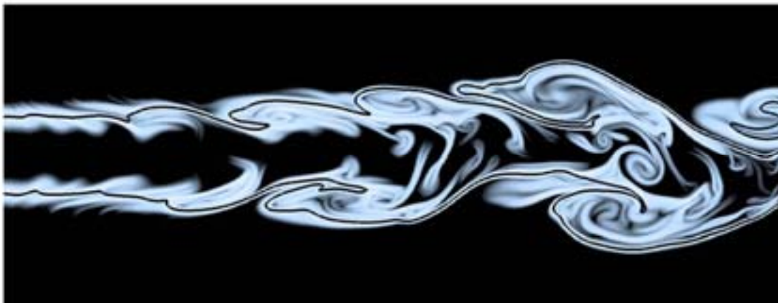
Figure I-1.4 Mixing in direct numerical simulation of a turbulent reacting CO/H 2 /N 2 jet flame as revealed by the scalar dissipation rate isocontours. The black isoline corresponds to the stoichiometric mixture fraction.
