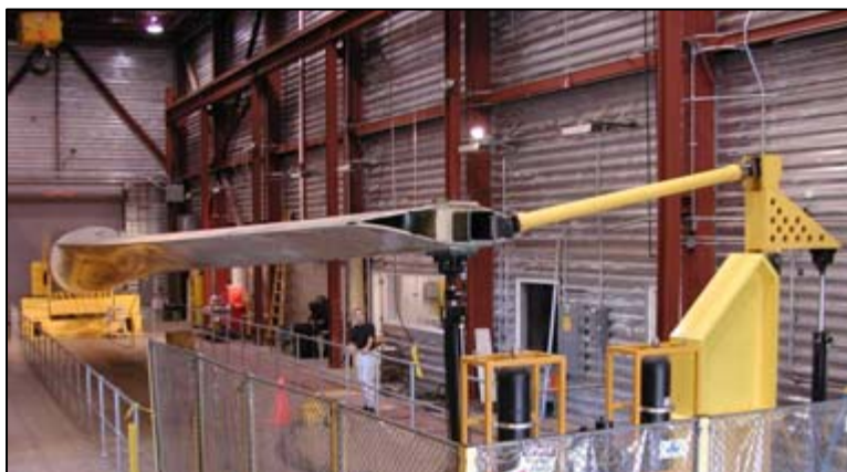
Figure 6: Bell crank system (painted yellow) used in the 34-m NWTC Blade Test Facility for edgewise fatigue testing
