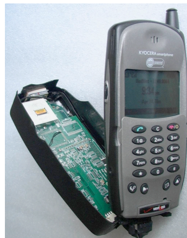
Fig. 5. The RadNet handheld cell-phone-based radiation system uses a low-power, pixelated cadmium-zinc-telluride detector to provide gamma-ray spectroscopy at low cost.
