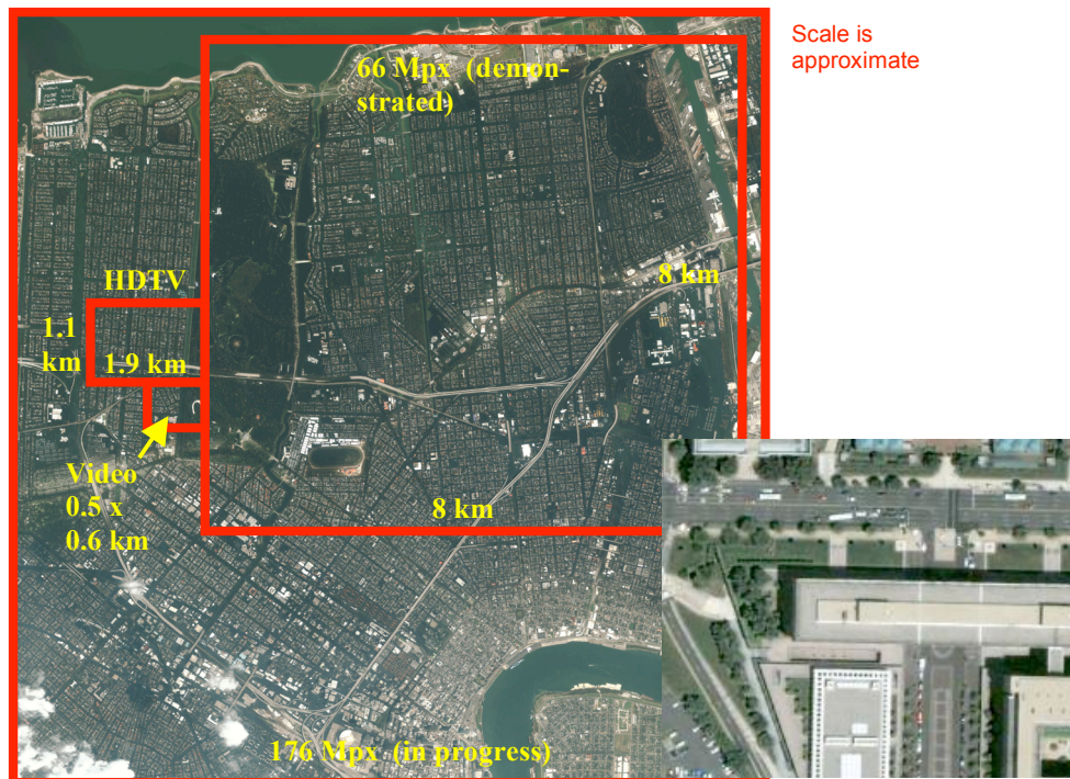
Fig. 7. Sonoma high-resolution, broad field-of-view coverage superimposed on recent satellite image of New Orleans flooding in the aftermath of Hurricane Katrina gives an example of the areal coverage associated with current and future sensor systems. The red squares show different fields of view for a given altitude provided by standard video, HDTV video, and different generations of Sonoma sensor systems. The inset on the lower left shows the approximate quality of the imagery anywhere in the full image data.
