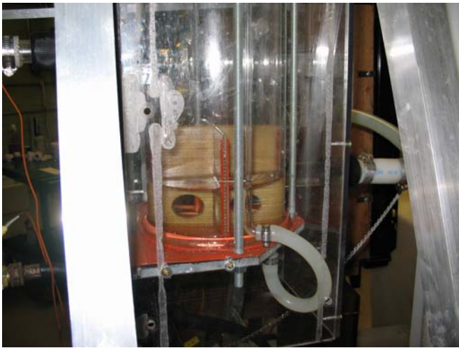
Figure 6 – Baffle Plates at Bottom of Glass Separator
