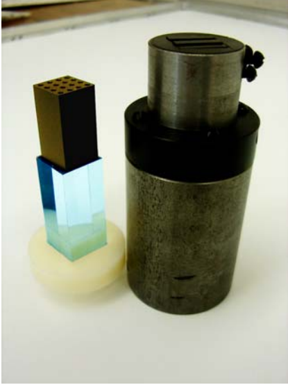
Fig.3. The template placed on top of the crystal (left) and a PMT housing head (right).
