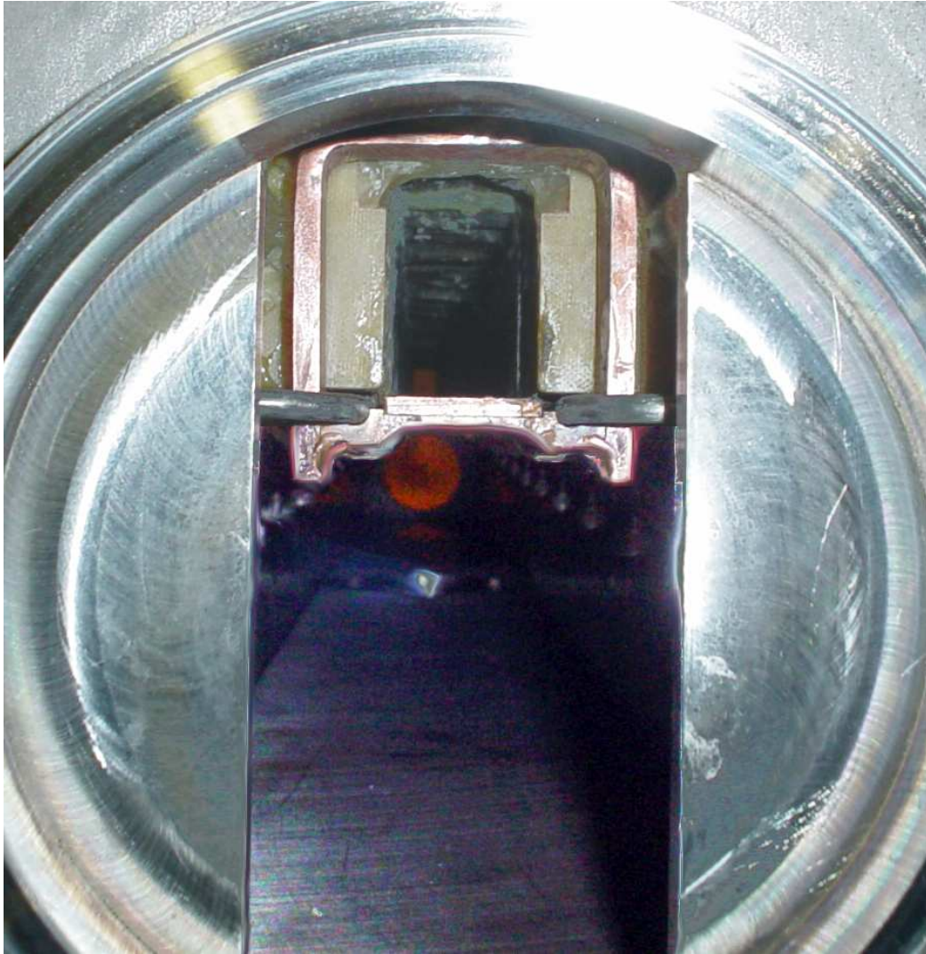
Figure 3.13: View inside a Booster extraction septum magnet. The circulating beam travels through the large horizontal region where there is no magnetic field. The extracted beam exits through the smaller aperture above the copper plate where the magnetic field is pulsed.
