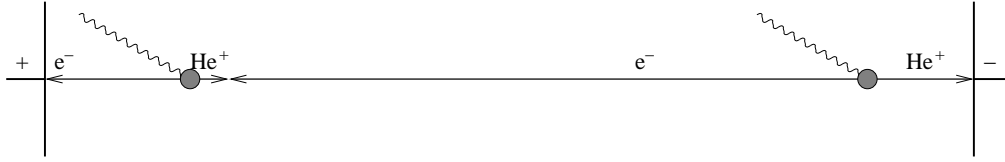
Figure D.4: Illustration of charge flow in the case of recombination.
