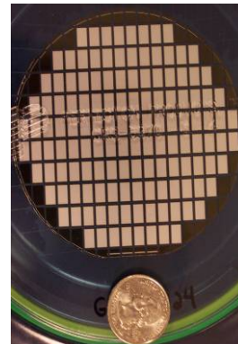
Fig. 3.14. 75-A Schottky diodes developed by Cree.
