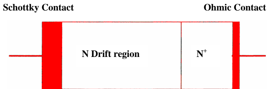
Fig. 2.1. Cross-section of a SBD.
