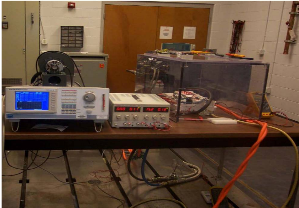
Fig. 3.20. Inverter dyne test setup.
