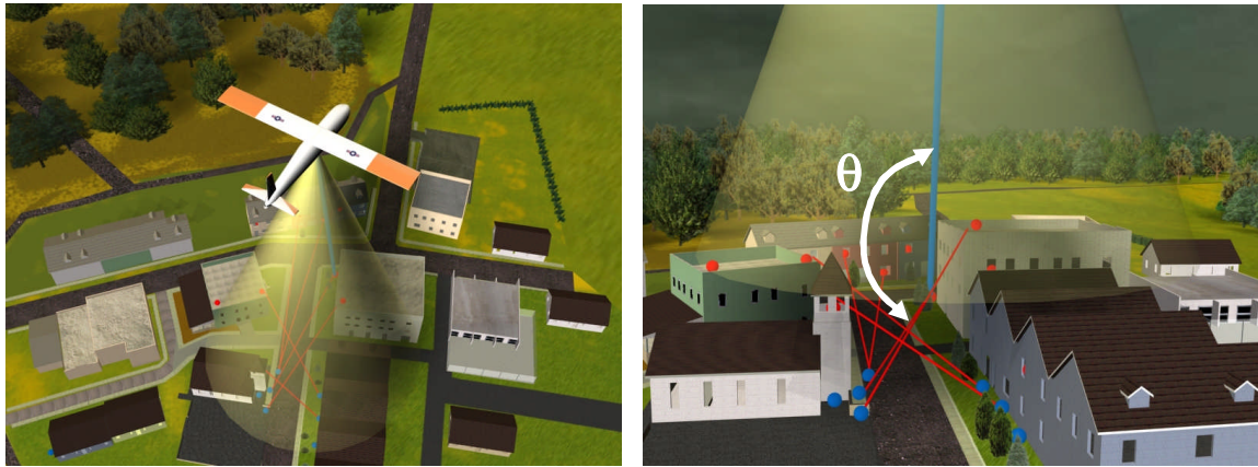
Figure 2. Illustrative FightSight UAV surveillance scenario with relevant sensor-to-shooter/shot-line angle \theta .
