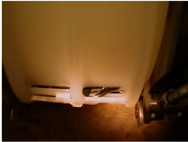
Figure 12. Sustained pressure testing to verify leak tightness of proposed seal design at 90 psig internal pressure
