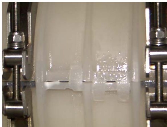
Figure 10. Sustained pressure testing to verify leak tightness of proposed seal design at 60 psig internal pressure
