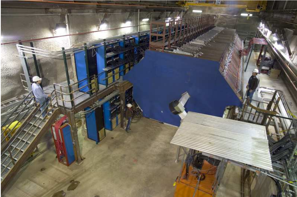
Figure 3.8: Photograph of the Near Detector (courtesy of Fermilab Visual Media Services). The racks along the left-hand side hold the electronics and the MA PMTs. The magnetic coil can be seen to extend from the front of the detector and drop diagonally down to the right side of the detector.
