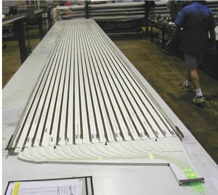
Figure 3.6: Photograph of an open scintillator module. The module is 20 strips wide. In the foreground is the manifold that guides the WLS fibres to the optical connector. The extra lengths of fibre within the manifolds are often referred to as “pigtailed”.
