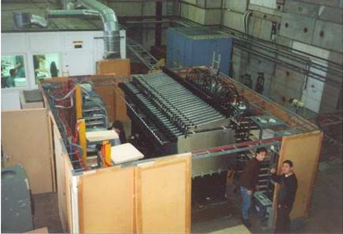
Figure 3.11: Photograph of the Calibration detector. The detector is shown during assembly in its enclosure outside of the test-beam. The alternating orientation of the planes can be seen.
