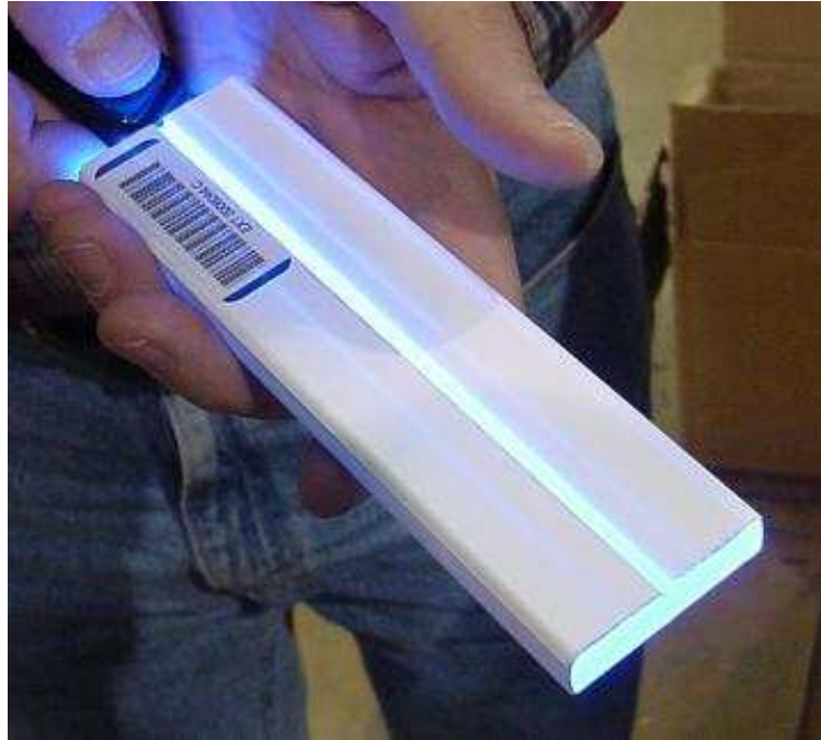
Figure 3.5: A short length of MINOS scintillator illuminated by a blue LED. The groove for the wavelength shifting (WLS) fibre can clearly be seen along the length of the strip. A thin reflective layer of \text{TiO}_2 , on the outside of the strip, is co-extruded with the scintillator to maximise the light collection.
