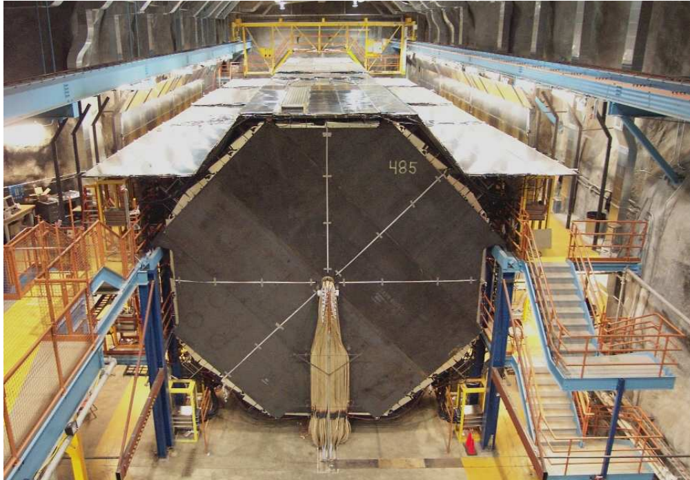
Figure 3.7: Photograph of the Far detector (courtesy of Jerry Meier). The magnetic coil can be seen to exit the centre of the detector and drop down to the floor. The scintillator planes on the top of the detector are a cosmic ray veto shield, vital for the atmospheric neutrino analysis.
