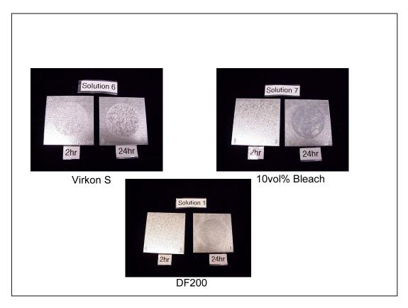
Figure 8: Photo comparison of galvanized steel surfaces after 2 hour and 24 hour exposures to Virkon S, 10vol% bleach and DF200.
