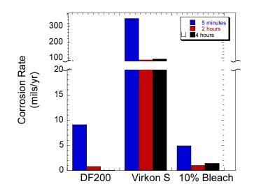
Figure 7: Corrosion rates of galvanized steel during exposure to DF200, Virkon S and 10vol % bleach determined by Electrochemical Impedance Spectroscopy (EIS).
