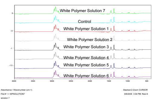
Figure 9: Spectra of white polymer material following exposure to various decontaminants.
