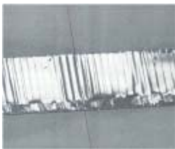
Fig. 6. Cut through the Hamamatsu MCP with the inclined holes, which is used in the tests of this paper. The MCP hole angle is 6.5^\circ .
