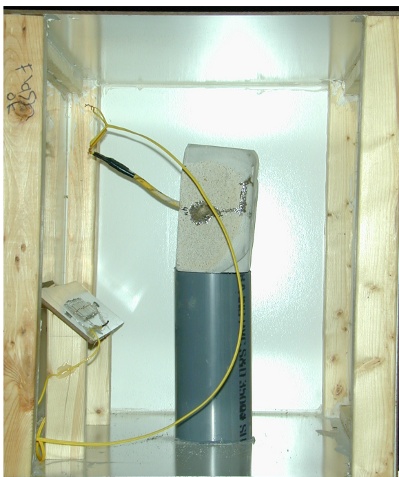
Figure 12. A test sample in its box with the flash array (left), and tied in to the initiator (yellow cord).
