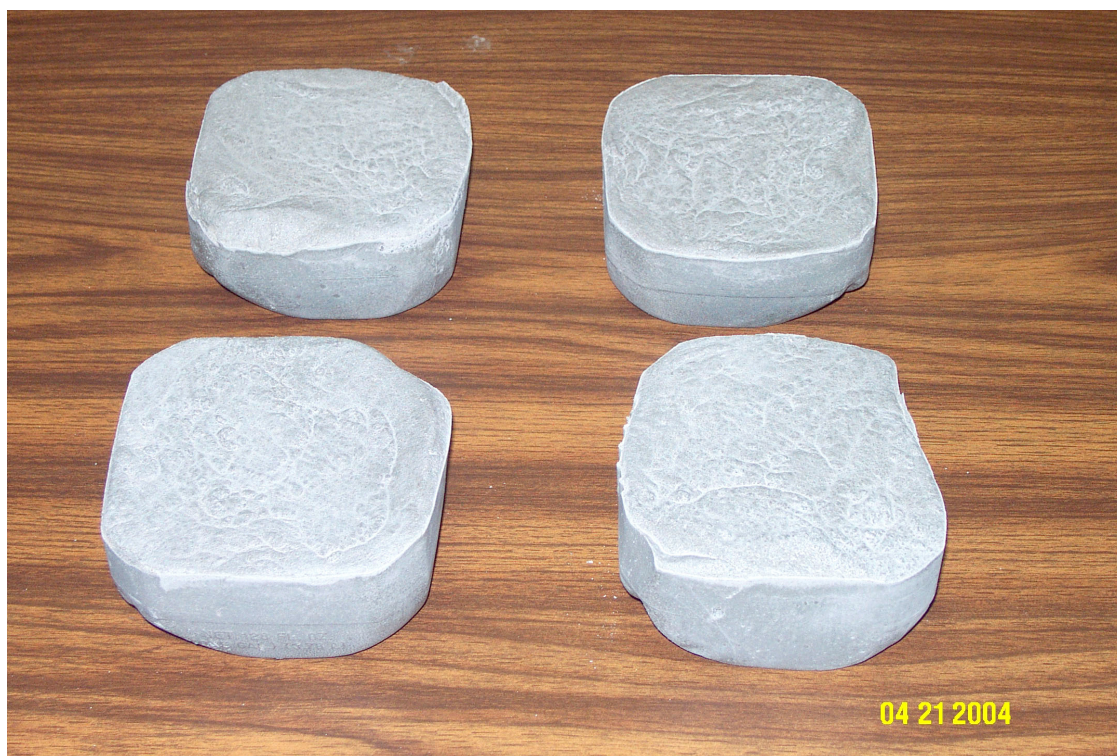
Figure 8. Preliminary mortar samples, after removal from molds.
