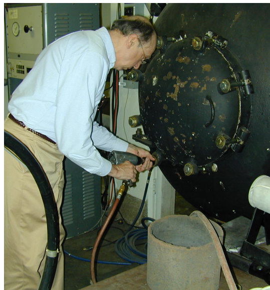
Figure 11. A test sample being loaded (left) and sealed (right) in the blast chamber.
