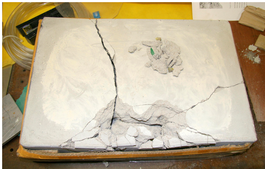
Figure 21. Test Sample 5 re-assembled after the shot. Loose fragments are piled at upper right.
