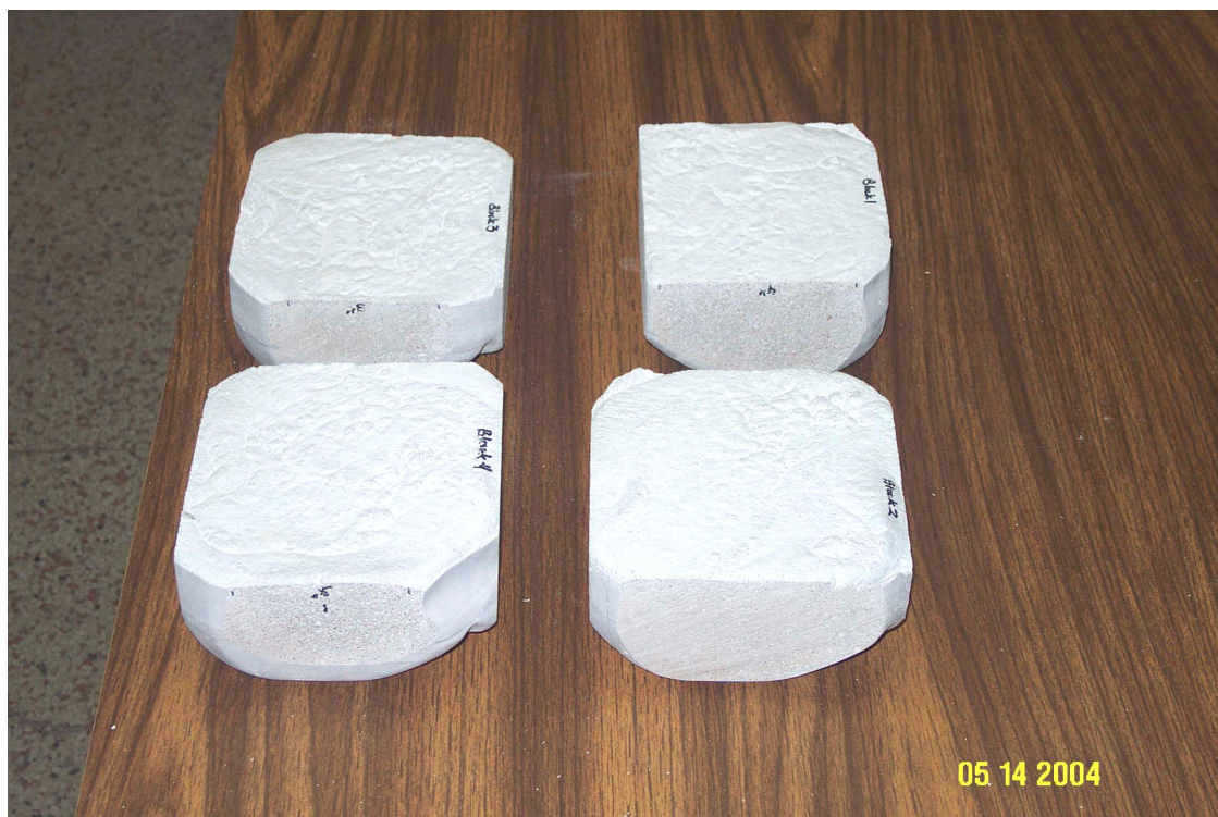
Figure 9. Preliminary mortar samples, after face machining.
