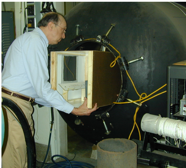
Figure 11. A test sample being loaded (left) and sealed (right) in the blast chamber.
