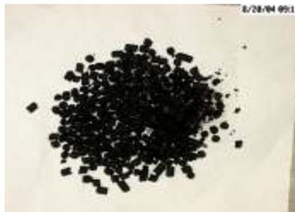
Figure 7 Char material produced by the Pyrolyzer
