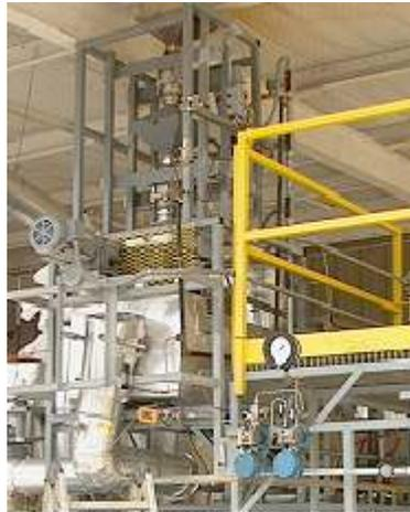
Figure 3 Pyrolysis Unit with Biomass feedstack system
