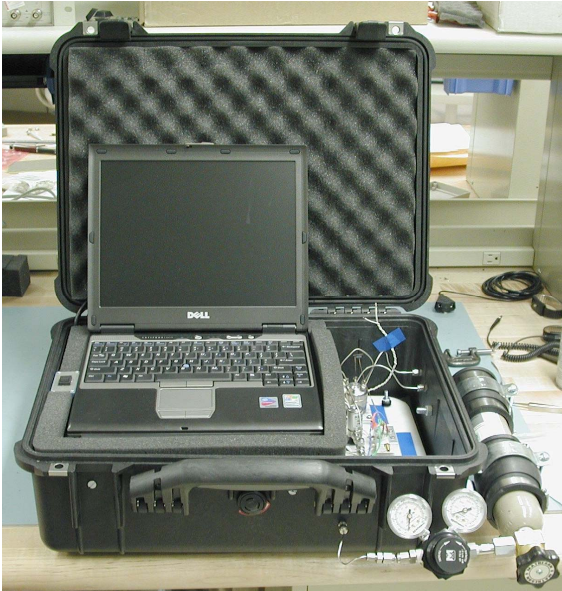
Figure 11. Field-portable natural gas analysis instrument. Chromatography hardware is visible to the right of the computer. Electronics boards are located under laptop.
