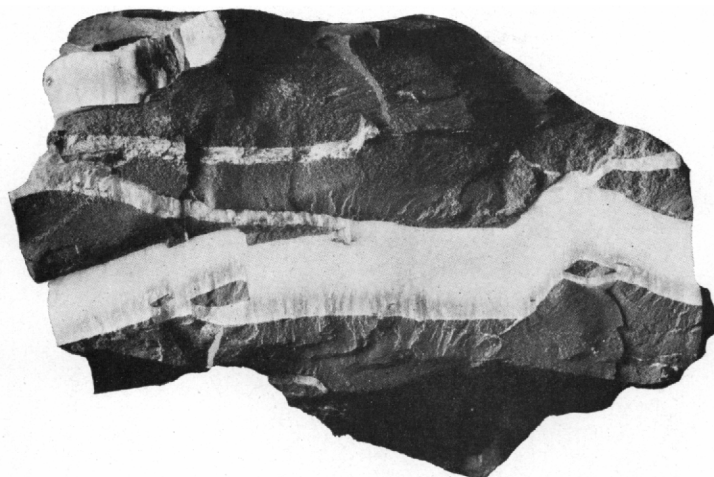
A. SEAMS OF ULEXITE IN CLAY ABOVE KERNITE DEPOSIT U. S. National Museum catalog No. 95831. Natural size.
