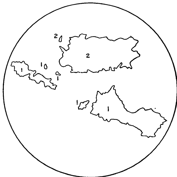
FIGURE 13.—Direct tracing of a photomicrograph of the granitoid facies of the quartz monzonite of the Pioche district, enlarged 32 diameters. Shows the remnants of two plagioclase grains in orthoclase, the replacement having been a deuteric effect. All outliers marked 1 extinguish together and were originally parts of a single large grain; the same for the outliers marked 2
