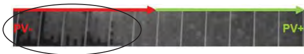
Fig. 1: High voltage stress degradation (PID) along module string in floating ground configuration [1]
