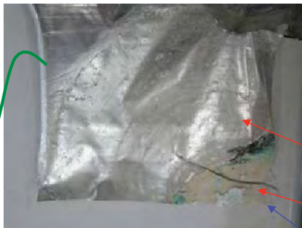
Inner Al layer of backsheet (EVA side)
