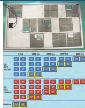
Figure 3: (a): Example of a harvested module (left) (b) Modules harvested at each time point for analysis and destructive testing (right)
