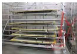
Fig. 5: Experimental setup 1 at Fraunhofer CSP with Al-foil covered PVC sheets
