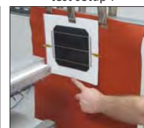
Figure 6: Soft backing test setup !
