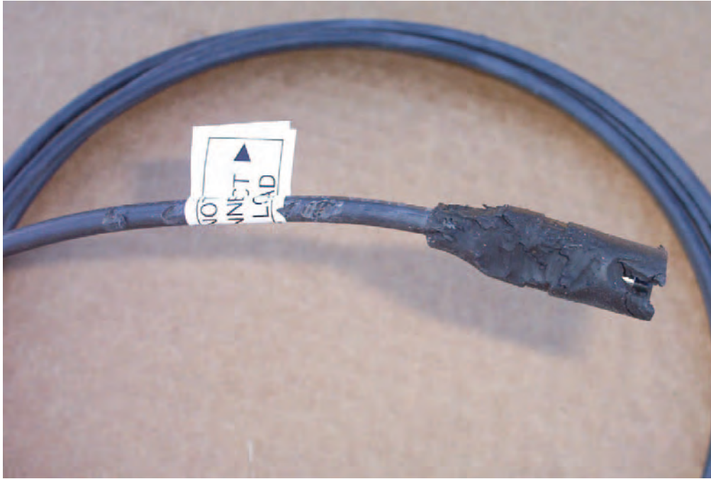
Photo #5 Chewing damage to a DC male connector (J. Wiles)
