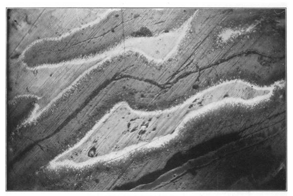
B. OXIDATION OF CHALCOPYRITE, O K MINE. Dark areas hydrous iron oxide, light margins undetermined sulphate?, light-gray areas unaltered chalcopyrite. Enlarged 180 diameters.
