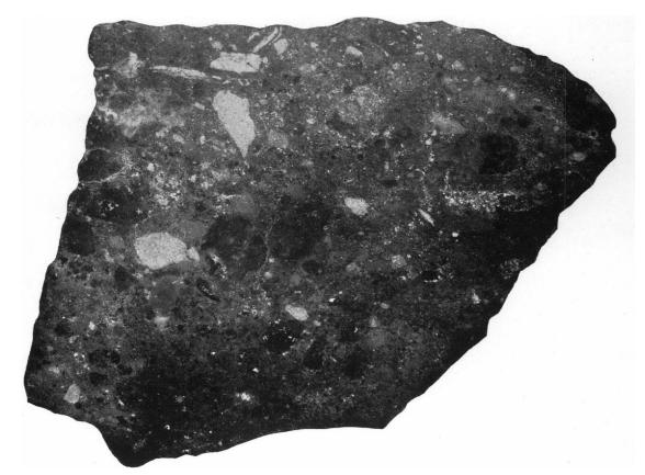
B. HIGH-GRADE ORE. BRECCIA ORE, HORN SILVER MINE. Light areas altered country rock, dark areas largely sulphides. Three-fourths natural size.
