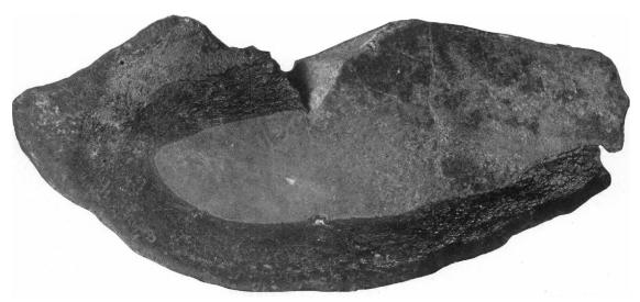
*B.* COVELLITE REPLACING ZINC SULPHIDES, HORN SILVER MINE. Zinc sulphides in the center, surrounded by zone of covellite containing considerable unreplaced zinc sulphide. Specimen collected by D. P. Rolfing.
