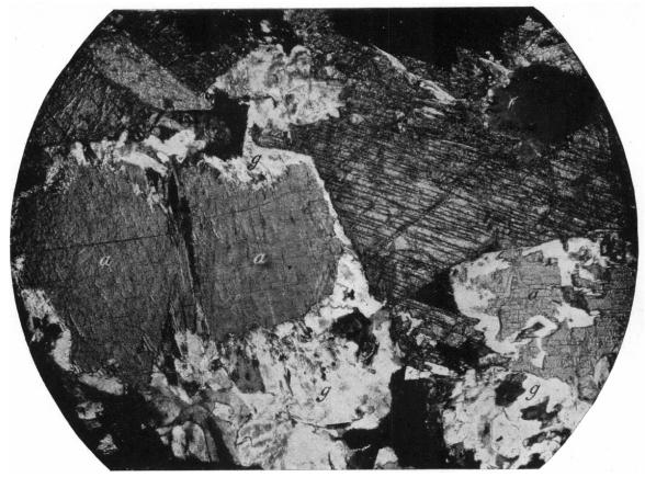
.1. ANHYDRITE ALTERING TO GYPSUM, CACTUS MINE. a, Anhydrite. g, gypsum. Enlarged 30 diameters.
