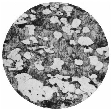
A. SERPENTINE IN LIMESTONE, NEAR CONTACT EAST OF MICHIGAN MINE. Probably alteration of diopside. The expansion in alteration has fractured the carbonate grains and the serpentine has filled the fissures. White areas serpentine, gray areas carbonate. Enlarged 30 diameters.
