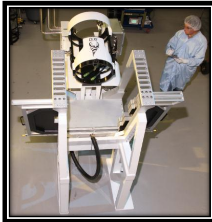
Figure 18. DIXI with 3x shield drawers installed for testing. Shown in the open position.
