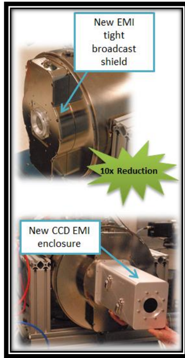
Figure 15. Updated Configuration with new integrated EMI broadcast shield and electronics
