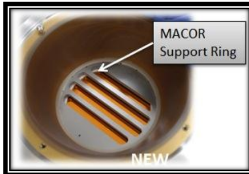
Figure 11. New photocathode shown installed in the DIXI with gold contacts, new Macor support frame and revised tensioning/bonding procedure
