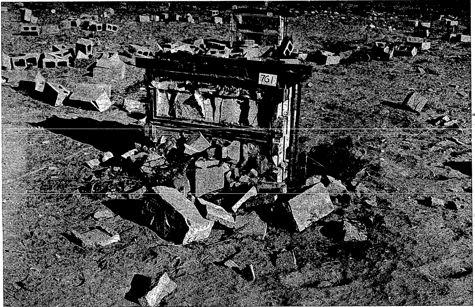
Fig. 6.72—Traps 7G1a and b (foreground) and 7G2a and b (background). The absorbers in the installation 7G1 traps, 10.2 ft behind the wall, were ruined by the impact of the large heavy blocks.
