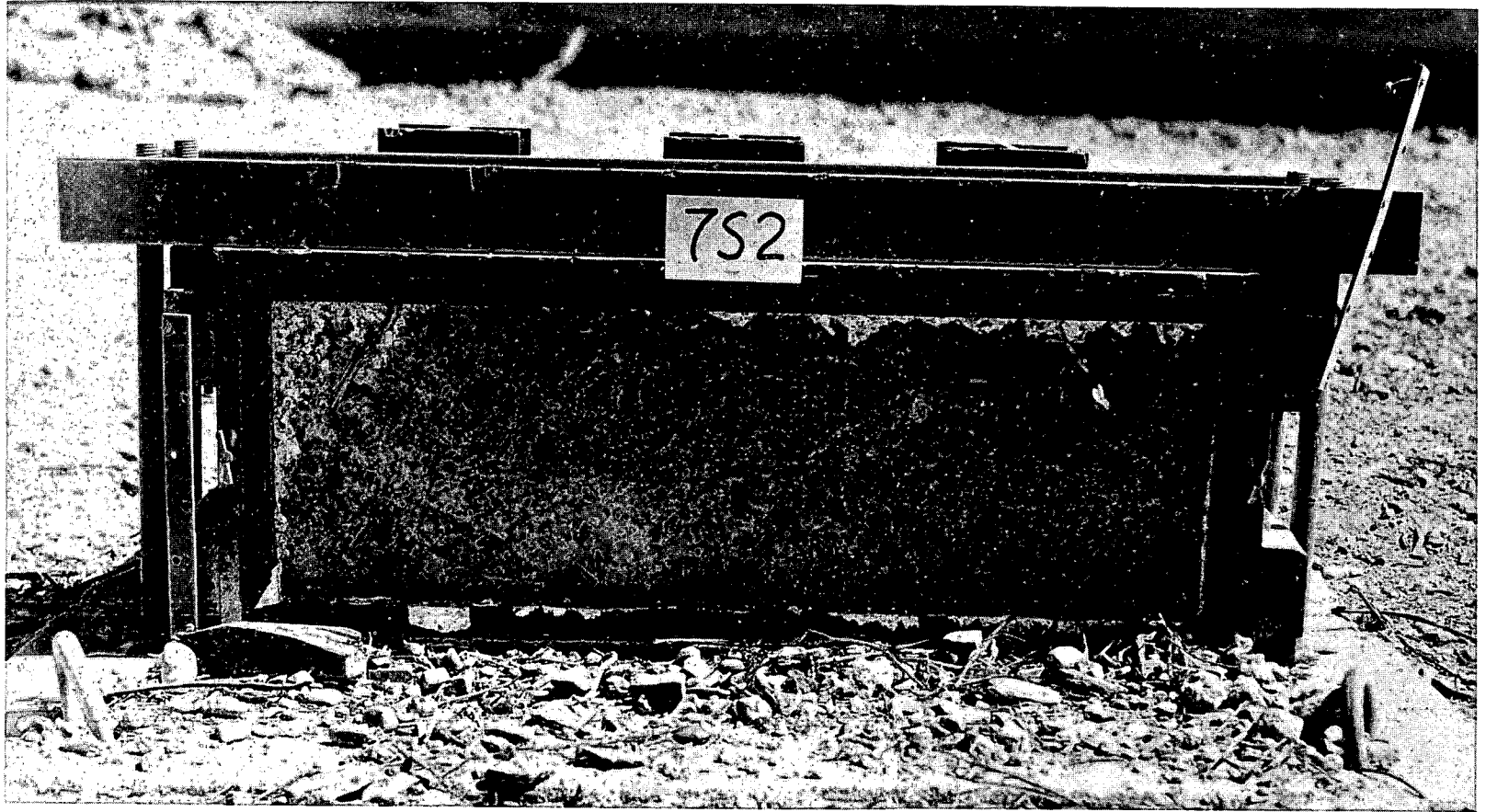
Fig. 5.47—Trap 7S2, postshot. A piece of the thermal-shield support can be seen on the right side of the trap.
