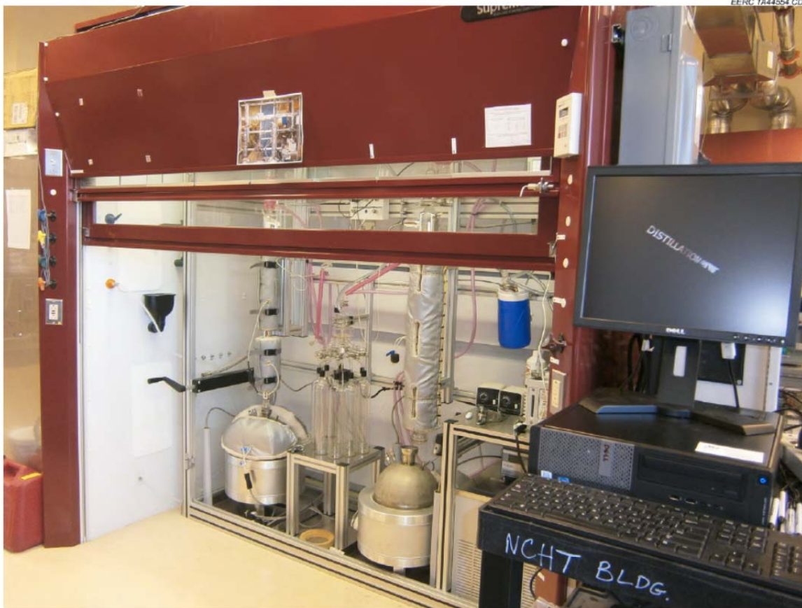
Figure II-11. Offline Distillation System at EERC
