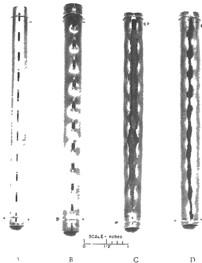
Figure 4 PHOTOGRAPH SHOWING TYPE 304 STAIN- LESS STEEL-CLAD URANIUM DIOXIDE FUEL ELEMENTS AFTER VARIOUS STAGES OF OXIDATION
