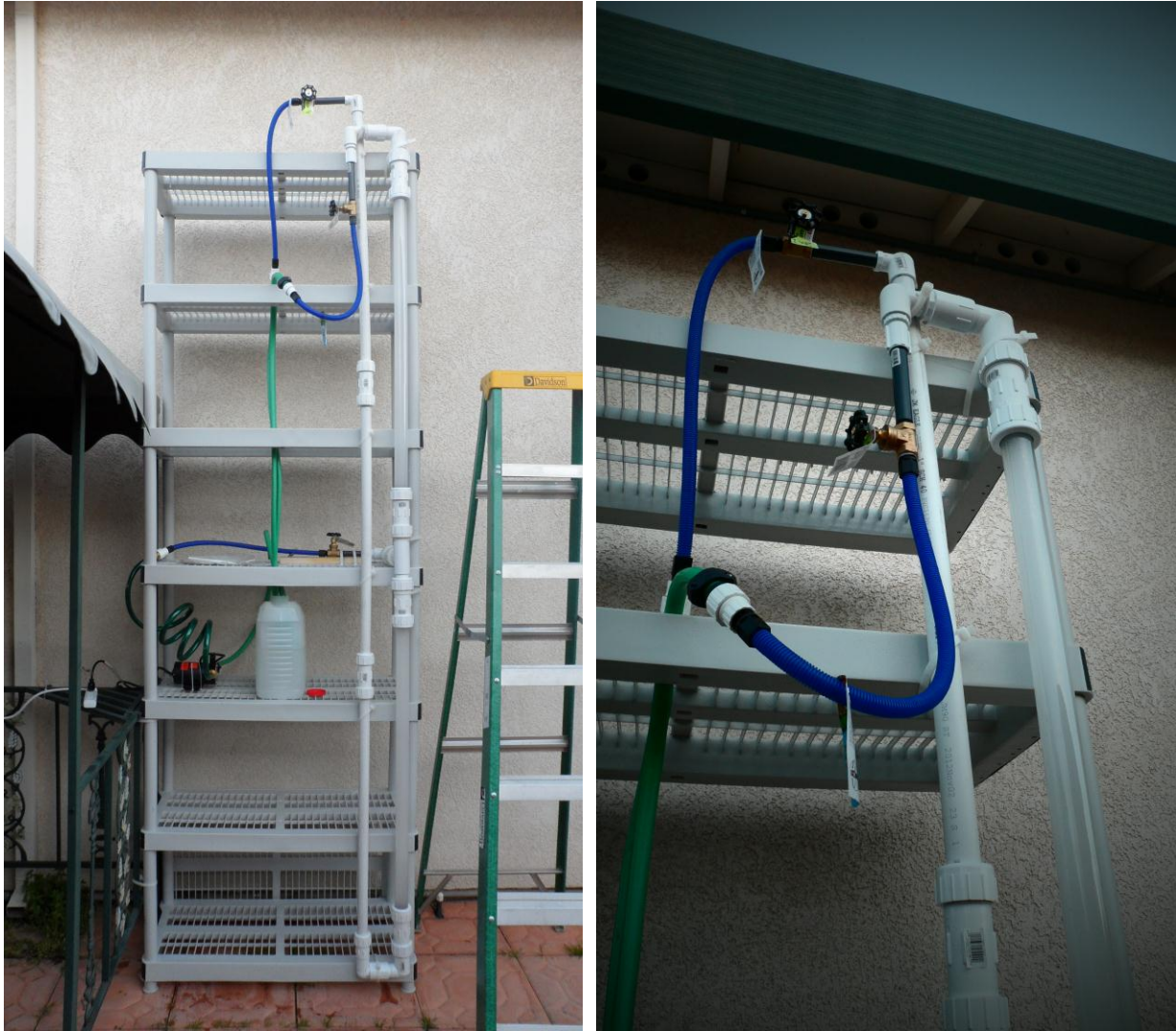
Figure 26 – The viability of using a hydro-cyclone for the separation of immiscible liquid phases has been demonstrated with both CFD models using COMSOL, as well as clear plastic models, as shown here. In this case, oil and water are separated in the hydro-cyclone (clear section of pipe on the right).
