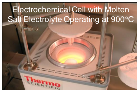
Figure 24 – High-temperature electrochemical cell at LLNL for proving the electrochemistry necessary for the halide-free alternative to Maroni tritium separation process, initially developed for high-temperature in-situ electrochemical studies of corrosion of LIFE chamber materials during exposure to high-temperature molten fluoride salts such as FLiBe and FLiNaK.
