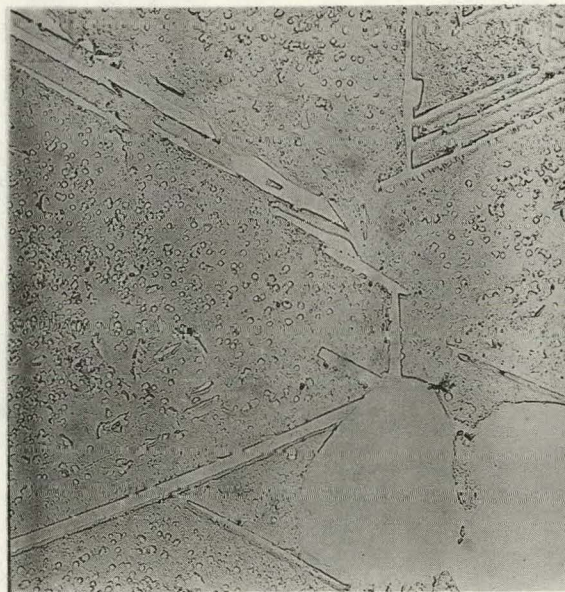
Fig. 14 Carbon replication showing Ni 3 Cb needles and possible Laves phase in material heated to 1,750°F (954°C) and cooled at 100°F (55°C)/hr.
