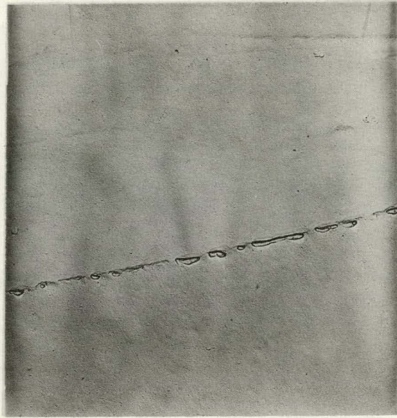
Fig. 15 Carbon replication showing possible CbC and M_6C at grain boundary in material heated to 2,000°F (1,093°C) and air cooled.
