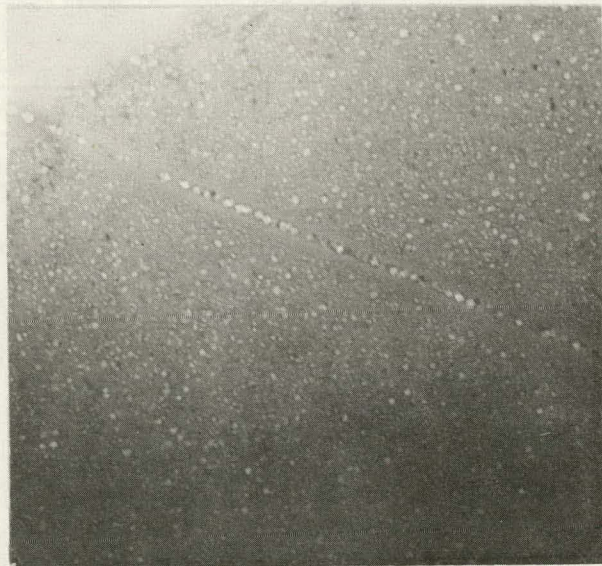
Fig. 16 TEM of material heated to 2,000°F (1,093°C) and air cooled, showing grain boundary denudation and possible CbC film in grain boundary.
