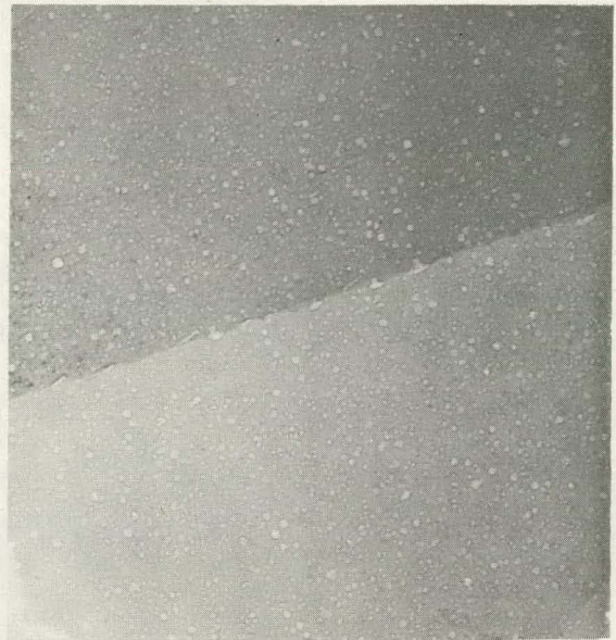
Fig. 10 TEM of material heated to 2,000^\circ\text{F} ( 1,903^\circ\text{C} ) and air cooled, showing hyperfine gamma prime.
