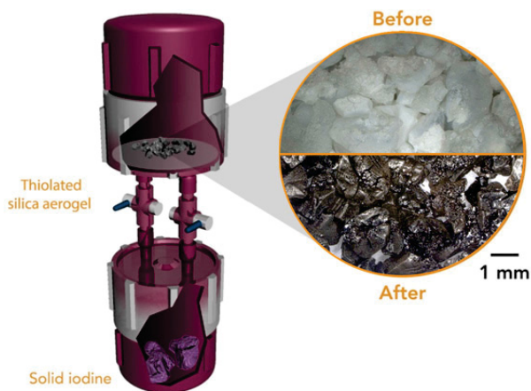
Figure 51. Assembly to determine iodine loading capacity of thiolated silica aerogel; iodine vapors at 150°C for 24 hr.
