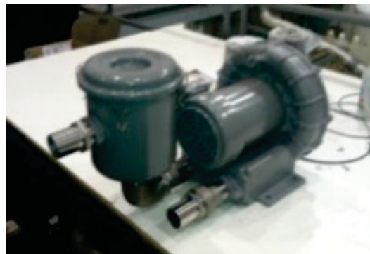
Figure 148. New exhaust blower.
