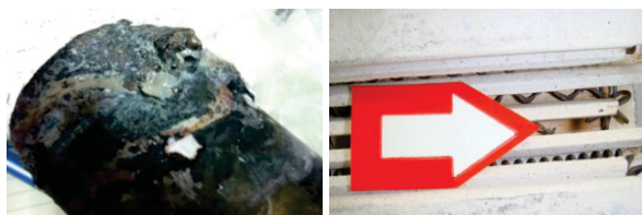
Figure 142. Observed damage to existing bottom drain tube and drain clamshell heater when exposed (for over an hour) at high temperatures (>1100°C) as required to melt solid crystals.
