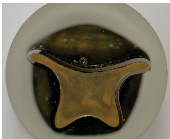
Figure 65. A photograph of the cross-sectioned HIP capsule containing iodine loaded Ag 0 Z
