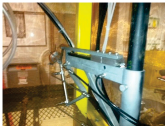
Figure 147. New CCIM Pilot Plant remote arm for graphite susceptor drain control and stopping with R, Z, and \Theta range
