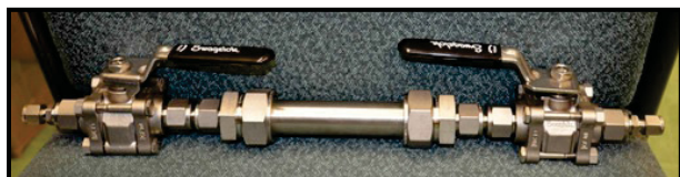
Figure 49: Test specimen holder for NO 2 aging of Ag 0 Z
