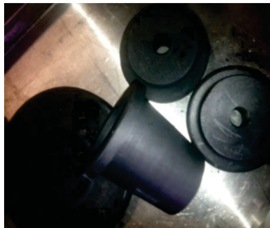
Figure 146. Different sized test specimens for the new crucible's graphite susceptor bottom drain tube.
