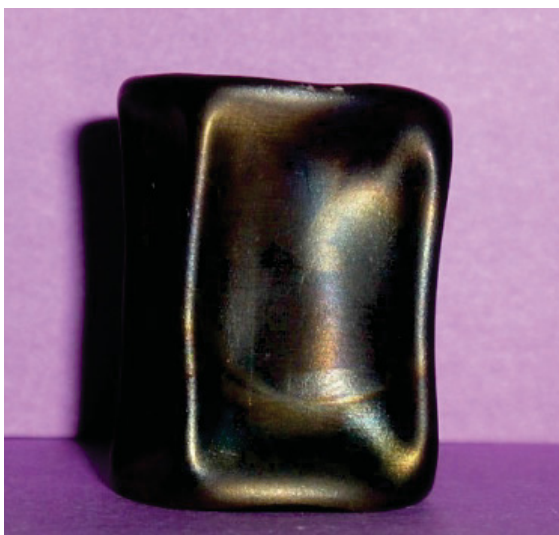
Figure 64. A photograph of the HIP capsule containing Ag 0 Z
