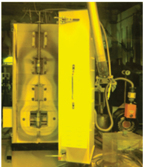
Figure 25. HFDA (top) and salt distillation apparatus/furnace (bottom) in the main cell of HFEF.
