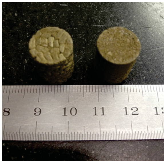
Figure 62. Compacts from pellet form Ag 0 Z (left) and crushed Ag 0 Z (right) after sintering in a HUP.
