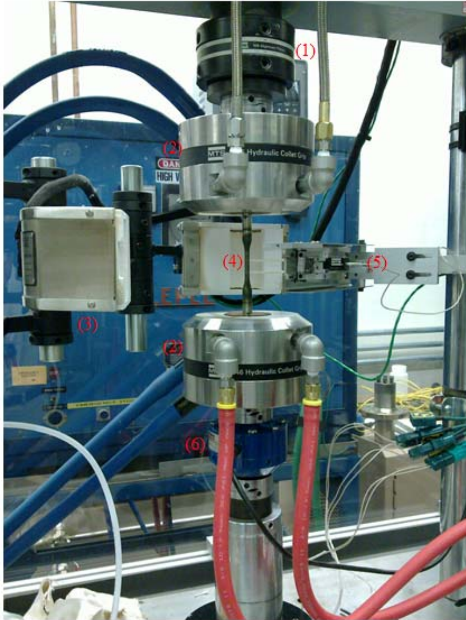
Fig. 3.14: Second set of creep-fatigue test frames. Detailed item description: (1) alignment fixture; (2) hydraulic grips; (3) furnace; (4) specimen; (5) high temperature extensometer; (6) load cell
