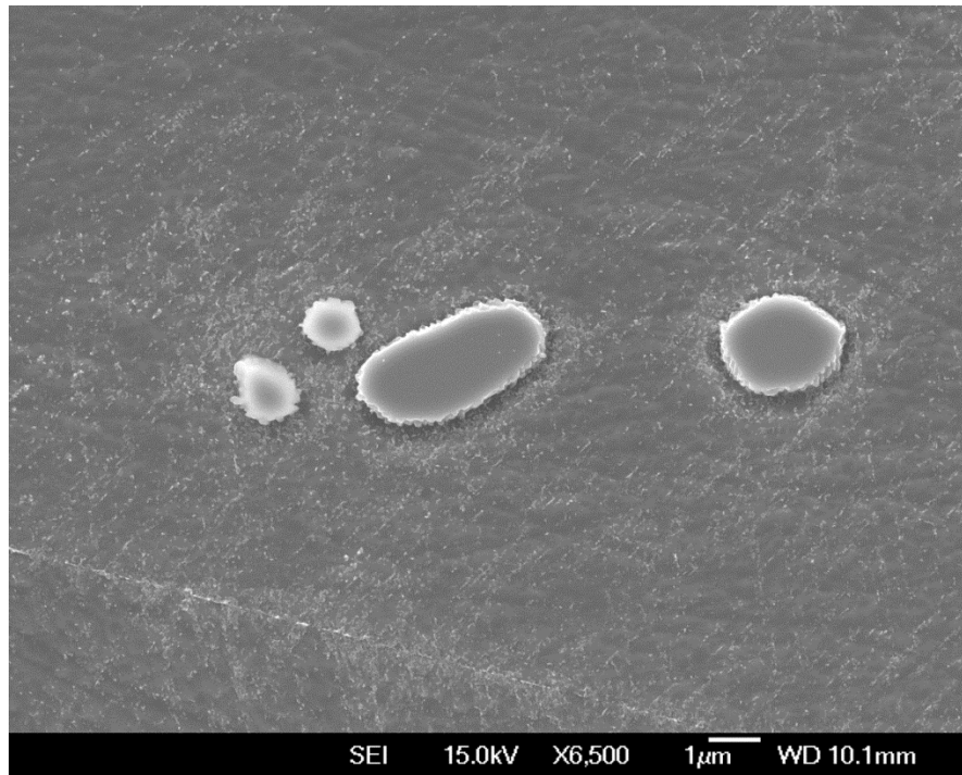
Fig. 4.81: Precipitation morphology on coherent and incoherent twinning boundaries of aged Alloy 617 specimens
