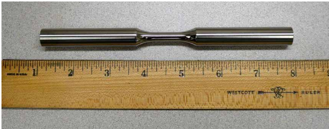
Fig. 3.11: Schematic for the straight-sided creep-fatigue specimen for hydraulic grips
