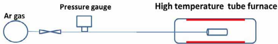
Fig. 3.19: The schematic diagram of creep tube testing performed at high temperatures
