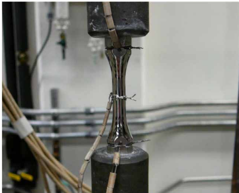
Fig. 3.15: Attachment of three S-type thermal couples to the specimen with Pt wires
