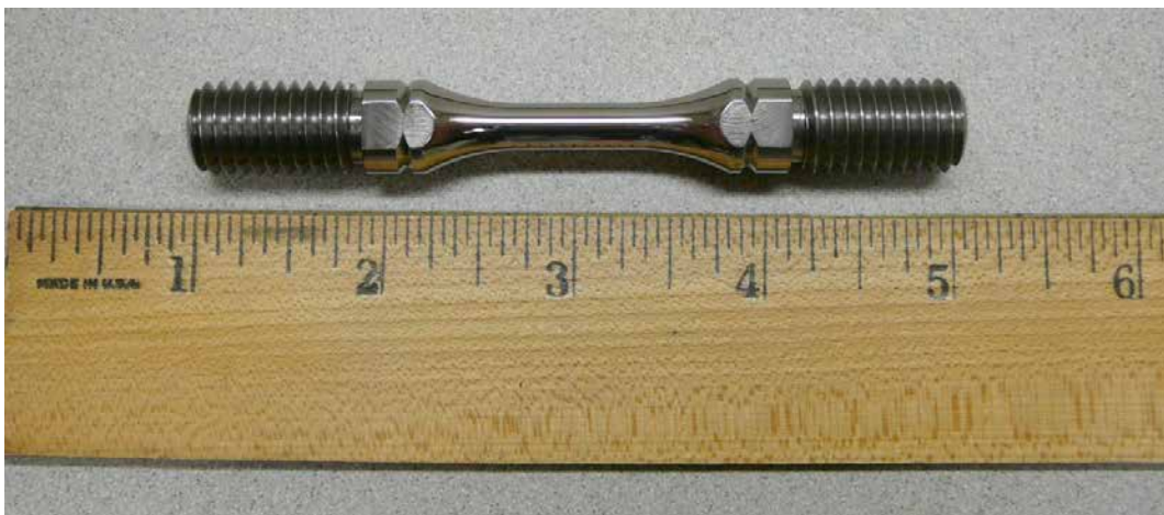
Fig. 3.12: Schematic for the threaded creep-fatigue specimen
