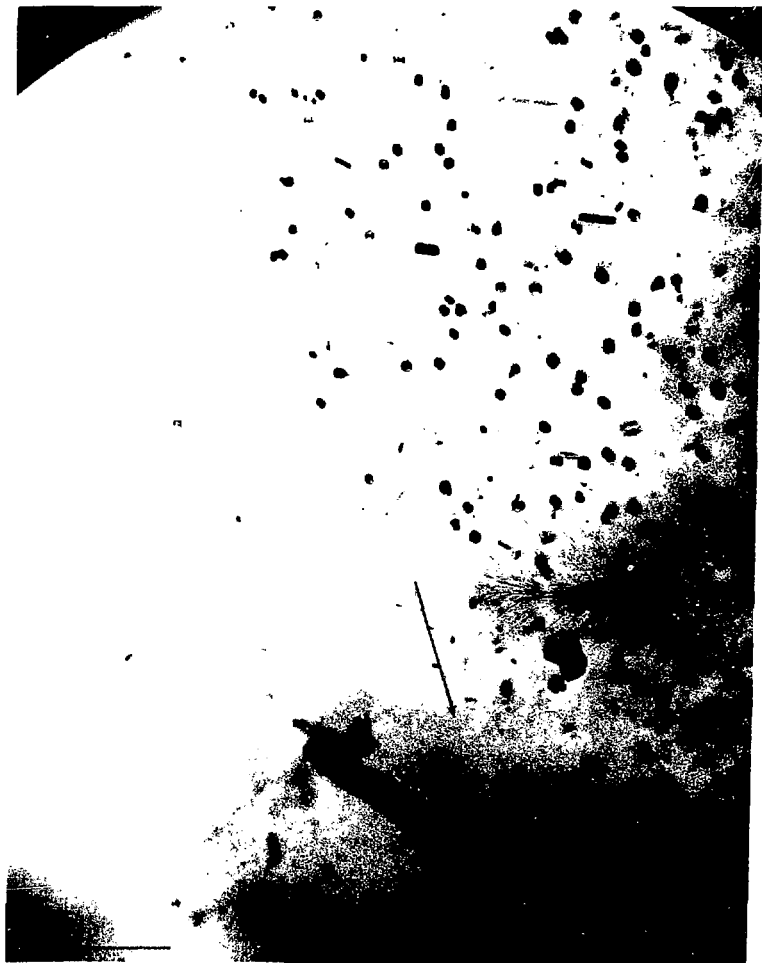
Fig. 4.12. Shows an area partially exposed to the ion-beam. Subsequent annealing shows that no defects form in the areas not bombarded. The possibility that furnace contaminants affect defects is eliminated.
