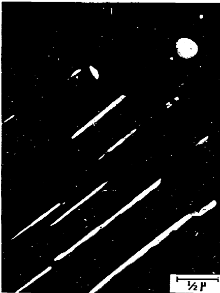
Fig. 17. Bright and dark field transmission micrographs illustrating diffraction by FeN precipitates at a depth of 0.025 in. after nitriding at 1310°C.
