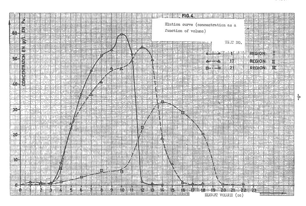
On the other hand, if the elution rate is such that the time of contact of the solution with the resin is less than the time necessary for establishment of the equilibriums of interest, the elution is controlled by the equilibrium kinetics and not by the elution rate (region II of Fig. 2). In other words, in this region the duration of the elution remains practically constant, while the eluant volumes necessary vary according to the rate.
